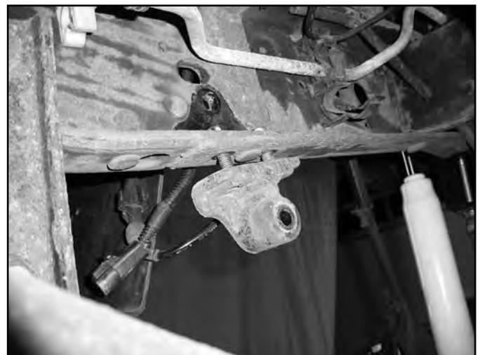
23. Reattach the front brake line brackets to the frame with the original bolts. Torque bolts to 15-20 ft-lbs.
