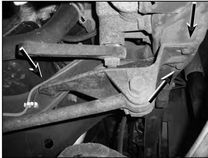
17. Install the new provided pitman arm on the steering sector shaft. Use the marks made on the factory arm as a guide. Fasten the pitman arm with the original sector shaft nut/washer. Torque nut to 185-200 ft-lbs.
