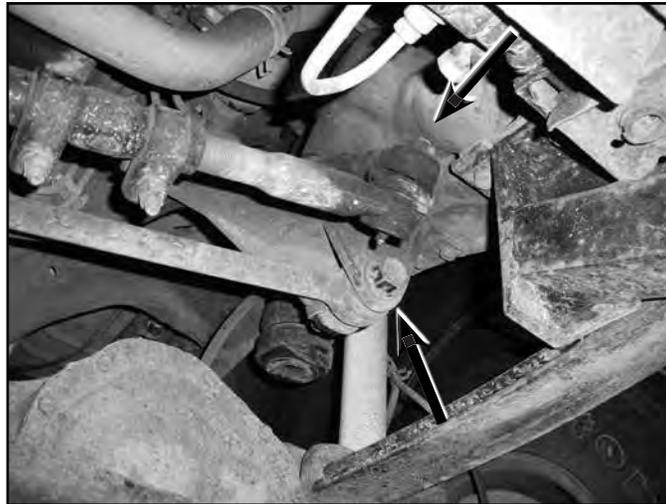
7. Remove the front shocks from the axle and frame mounts. Save hardware and discard shocks.
