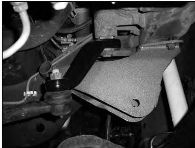
19. Remove the factory front bump stops from the frame rails (Fig 8). Locate the provided rectangle bump stop spacers (01027) and place between the factory bump stops and the frame rail. Align the holes in the bump stop and spacer with the original frame mounting holes and fasten with the provided 10mm x 110mm bolts and washers (BP 441) into the captive nuts in the frame (Fig 9) . Use Loctite on the bolt threads and torque bolts to 30 ft-lbs.
