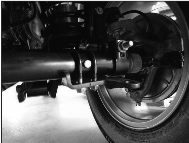
9. Loosely attach the passenger side stabilizer bracket to bottom side of tie rod link similar to the driver side with the provided 5/16" U-bolts, washers, and nuts. Leave hardware loose. Bolt Pack 304
