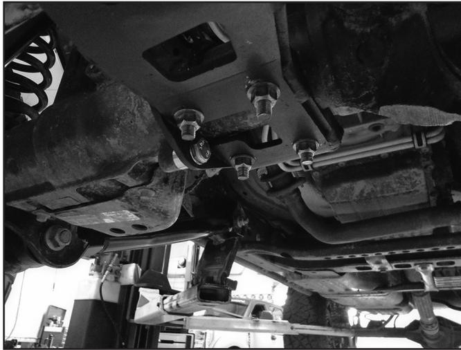
8. Attach the driver's side stabilizer bracket to the bottom side of the tie rod next to the clamp (Fig. 2) with the provided 5/16" U-bolts, washers, and nuts so the stabilizer mounting hole offsets to the outside. Leave hardware loose. Bolt Pack 304
