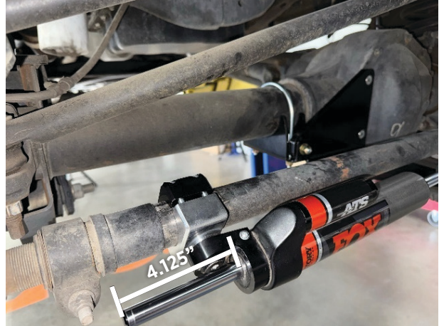
Fig. 16: Attach the stabilizer to the tie rod with the clamp.
