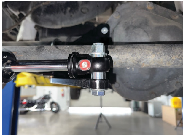
Fig. 17: Attach the stabilizer eyelet to the L-bracket; torque the nyloc nut (85 ft-lbs).
