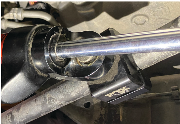
Fig. 2: Loosely clamp the stabilizer to drag link.
