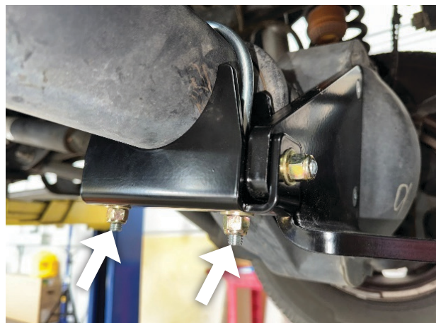
Fig. 15: Torque the nyloc nuts (30 ft-lbs); ensure exposed threads are equal on both sides.
