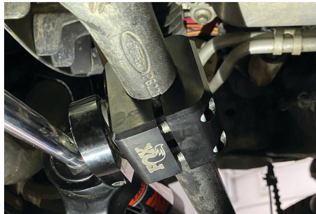
Fig. 3: Use the supplied screws to mount clamp.
