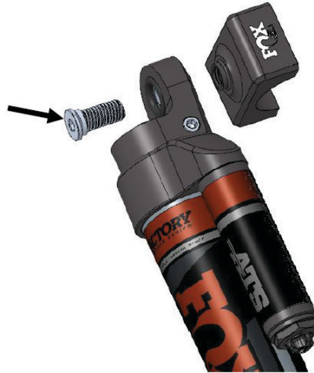
Fig. 6: Apply high-strength thread lock and torque to 30 ft-lbs (Hardware C1 & C2).
