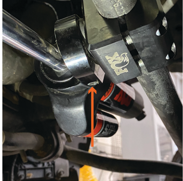
Fig. 5: The pinch bolt is located on L-bracket.
