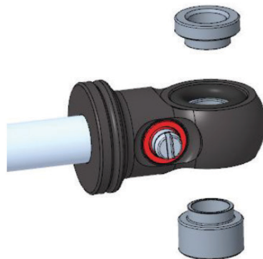
Fig. 7: Install reducers with the taller reducer on the bottom (Hardware F2 & F3).
