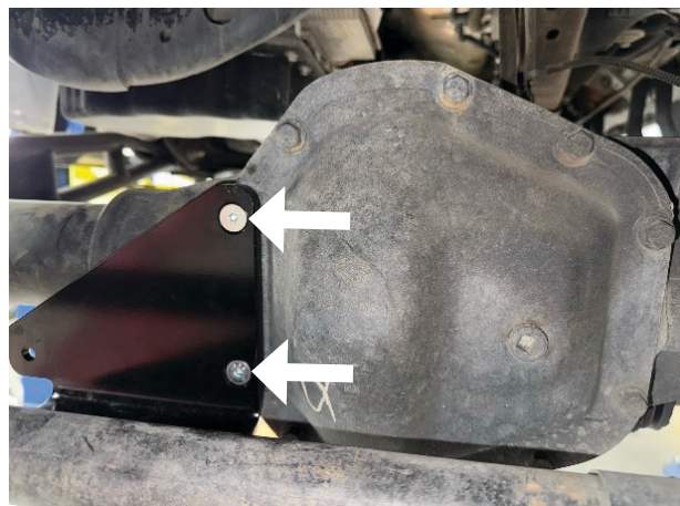
Fig. 12: Install the correct differential cover hardware for your vehicle.
