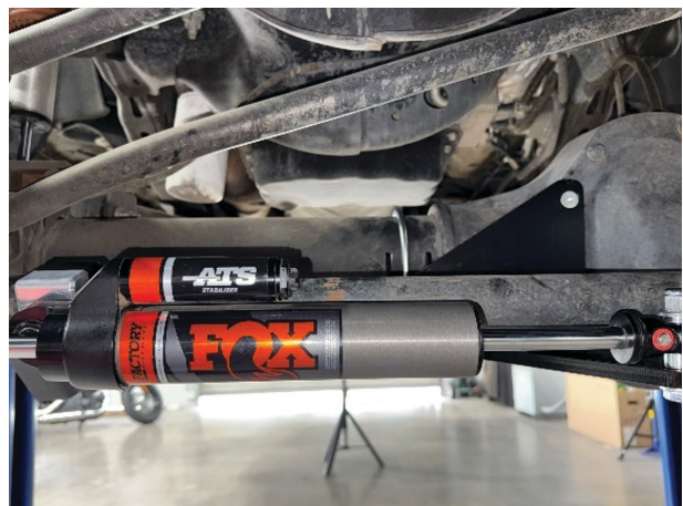
Fig. 18: Stabilizer in-line with tie rod.
