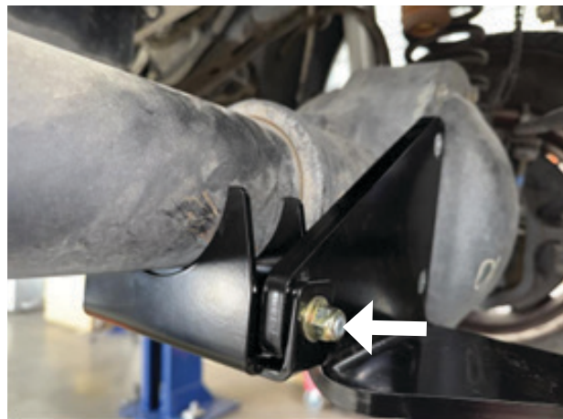
Fig. 14: Torque the nyloc nut (35 ft-lbs); ensure the U-bolt sits flush against the axle.
