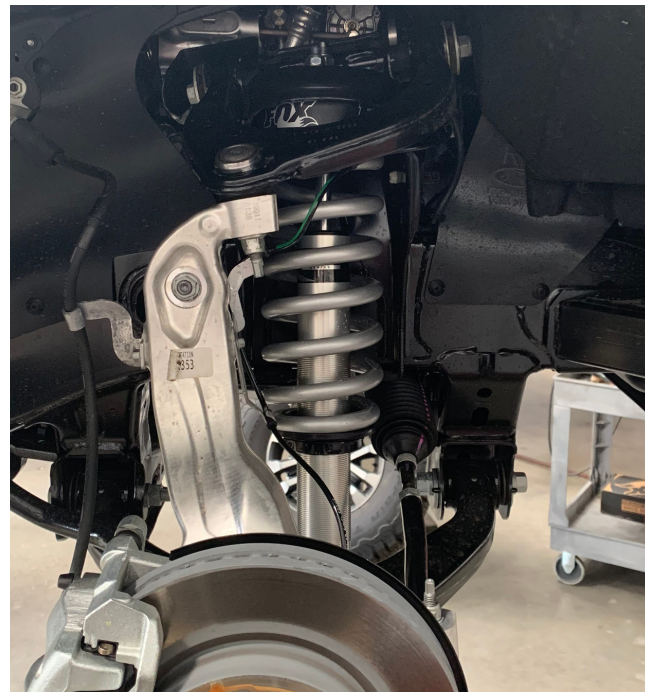
Fig. 14b: Passenger side shown. 2.0 Performance Series IFP shock
