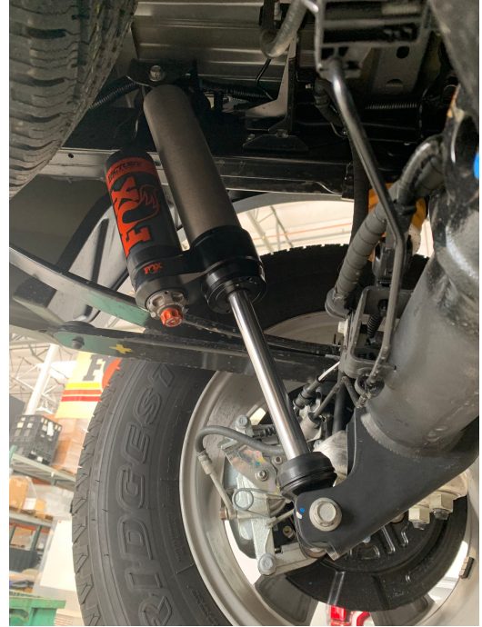
Fig. 15a: Driver side shown. 2.5 Performance Elite Series shock
