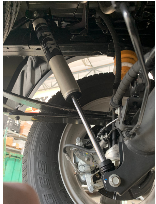
Fig. 15b: Driver side shown. 2.0 Performance Series IFP shock
