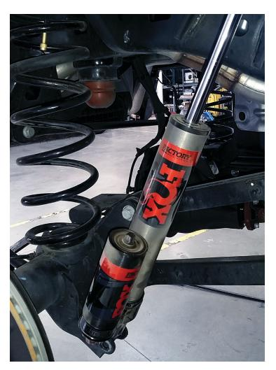
Fig. 6: Passenger side shown (2.5 Performance Elite Series model).
