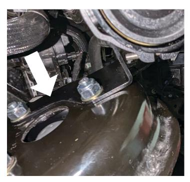
Fig. 3: External reservoir mounting bracket. Passenger side shown.
