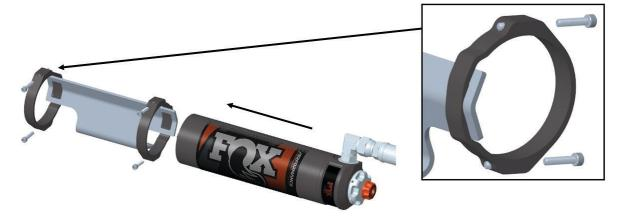
Fig. 5: Diagram of reservoir and bracket interface.
