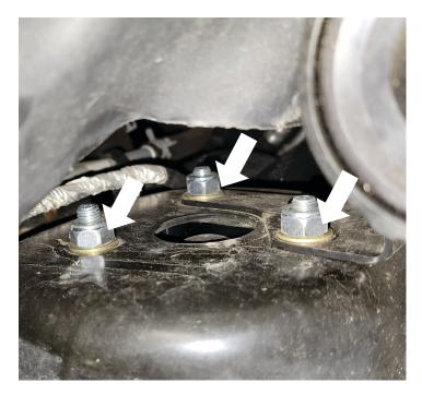
Fig. 4: Mounting bracket bolts. Passenger side shown.
