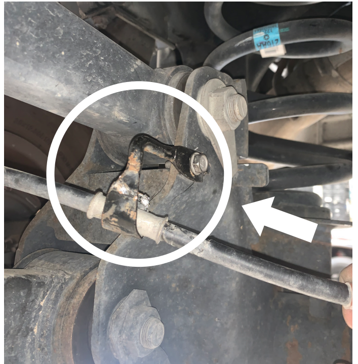
Fig. 4: Remove parking brake line (RAM 2500 passenger side shown)
