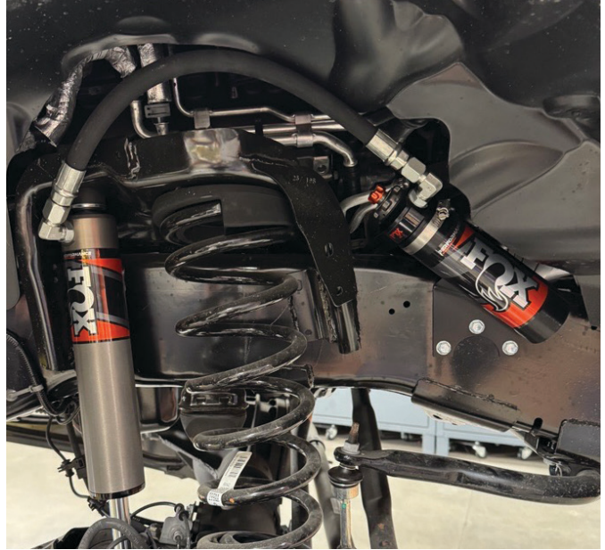
Fig. 1: Hoses facing outward and reservoir toward front of vehicle (passenger side shown)
