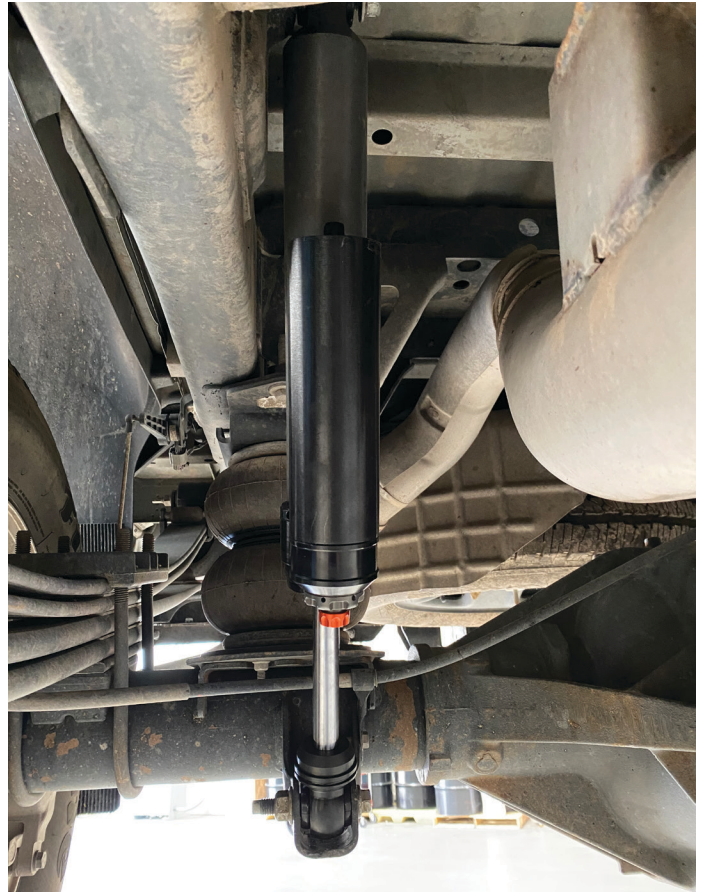
Fig. 8: Install FOX shock (RAM 3500 passenger side shown)
