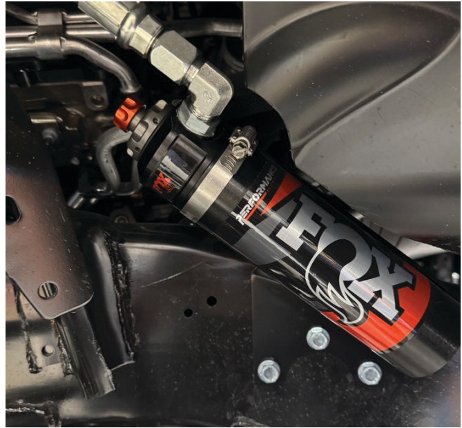
Fig. 3: Mount reservoir to bracket (passenger side shown).
