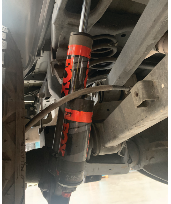
Fig. 6: Install FOX shock (RAM 2500 passenger side shown)
