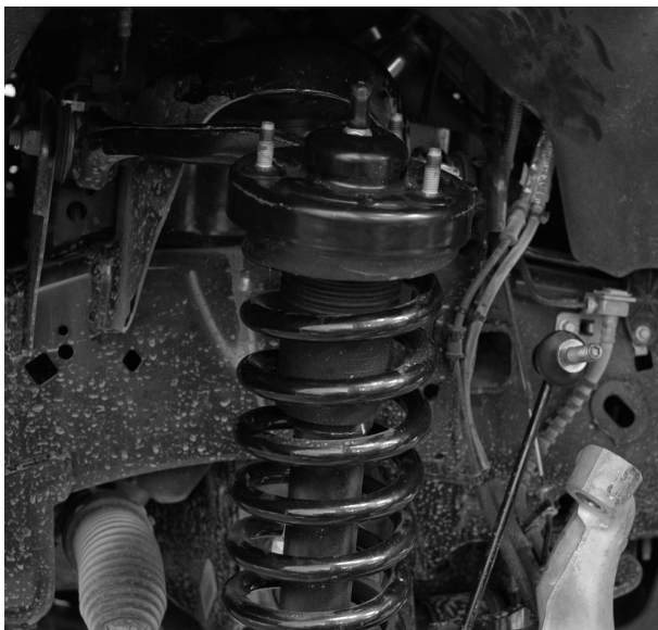
Fig. 6: Free the coil-over.
