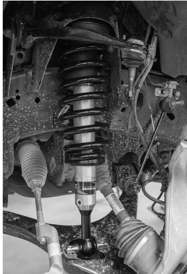
Fig. 14: Install the coil-over.
