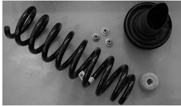
Fig. 10: OEM spring and associated hardware.
