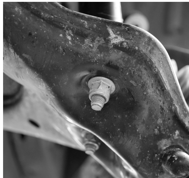
Fig. 7: Remove the bar-pin bolts.
