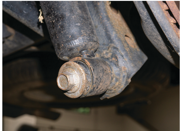
Fig. 21: Remove lower shock mount bolt.
