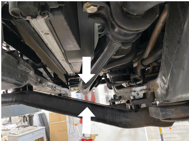
Fig. 16: Check clearance of the sway bar.
