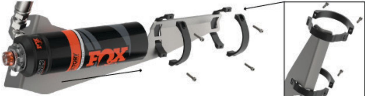
Fig. 10: Diagram of reservoir and bracket interface.
