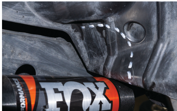
Fig. 25: Cut the fender liner.
