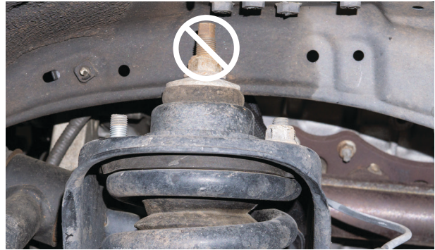
Fig. 4: Remove the three top hat nuts.
