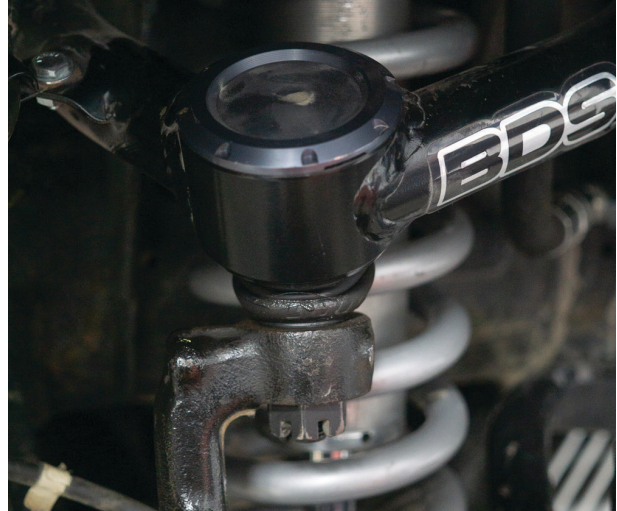
Fig. 7: Reattach UCA to the upright.
