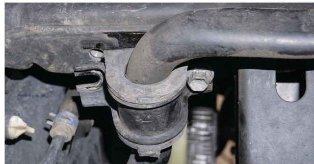
Fig. 11: Remove sway bar bracket.
