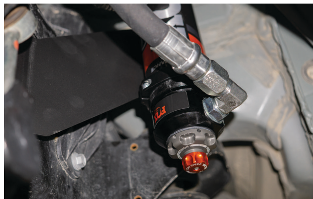
Fig. 22: Mount the reservoir to the bracket (passenger side shown).
