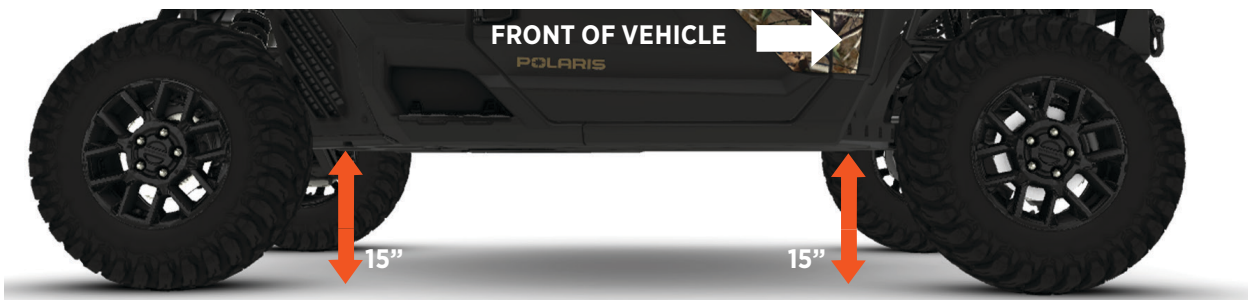
Fig. 2: Vehicle ride height: Front - 15\", Rear - 15\"
