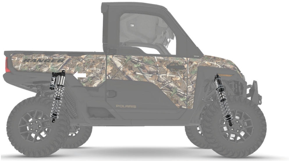
Fig. 1: Rear shock reservoirs point away from the cab. Front shock reservoirs point outward.
