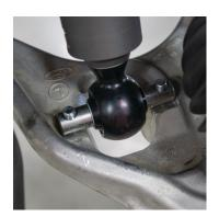
Fig. 18: Fasten the bar-pin bolts.
