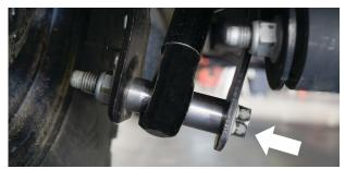
Fig. 29: The larger spacer mounts on the inboard side of the eyelet.
