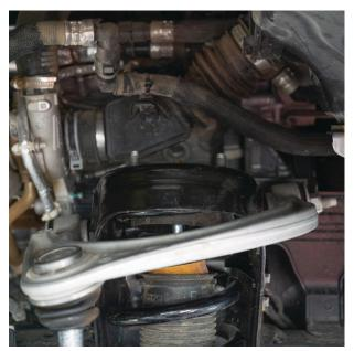
Fig. 7: DO NOT remove the center nut.
