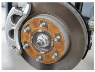
Fig. 20: Fasten the axle nut.
