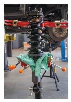
Fig. 15: Align the marks on the top hat and spring
