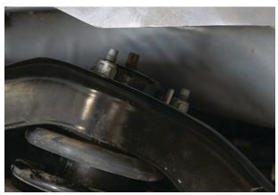
Fig. 26: Do not remove the center nut.
