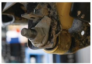
Fig. 25: Loosen the lower mounting bolt.
