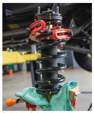
Fig. 11: Use a professional spring compressor.
