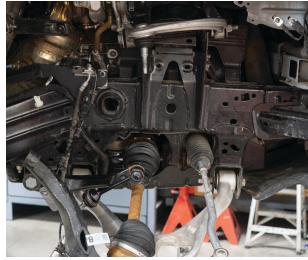
Fig. 9: Take off the bar-pin bolts.
