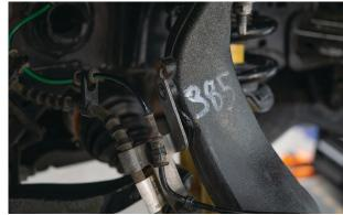
Fig. 1: Disconnect brake line bracket.
