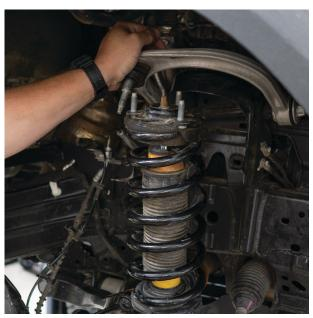
Fig. 8: Free the coil-over from the coil bucket.
