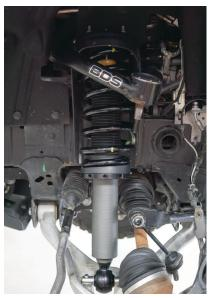
Fig. 16: Align marks on the coil bucket and top hat.
