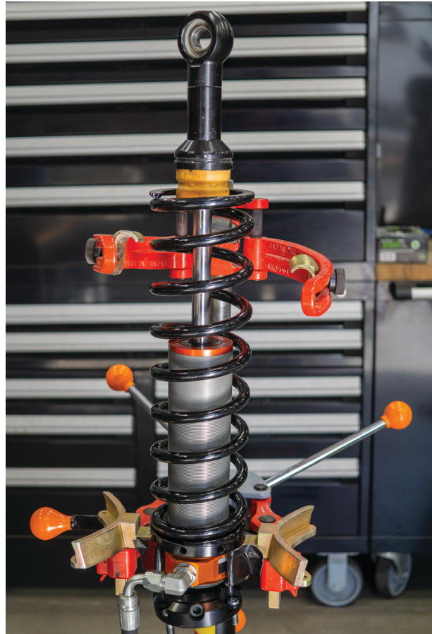
Fig. 4: Back off spring tension.
