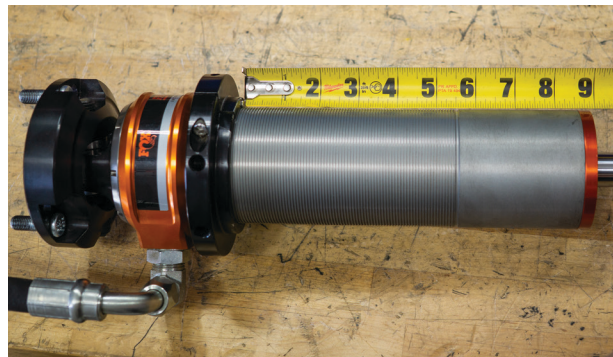
Fig. 5: Turn the preload ring until no threads show.
