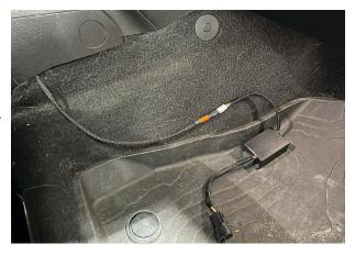
Fig. 10: Connect Controller to Switch Harness.
