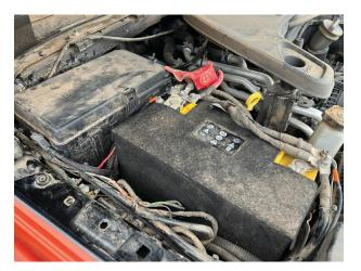
Fig. 30: Connect battery ground cable and GND\_BATTERY ring terminal.
