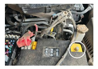
Fig. 17: Disconnect negative terminal on battery.
