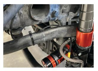
Fig. 23: Route the driver side Link Harness.
