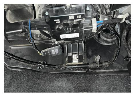
Fig. 15: Install harness in passenger footwell.
