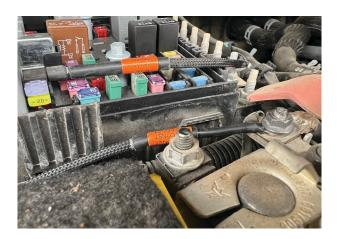
Fig. 28: Install the Micro3 tap into the lower slot and the 5A fuse into the upper slot; install Micro3 tap into empty slot for fuse #F52; connect two terminals.
