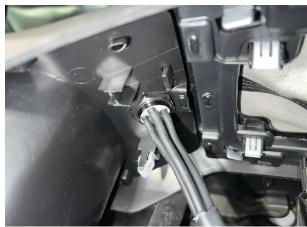
Fig. 8: Secure the switch in place.
