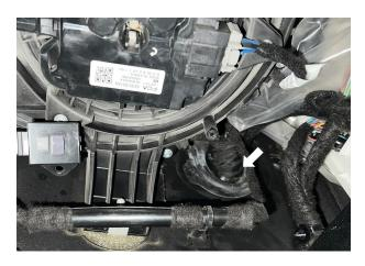
Fig. 14: Cut a slit in the OEM firewall grommet.
