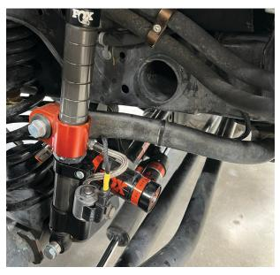
Fig. 21: Route the passenger side Link Harness.
