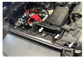
Fig. 19: Route the Link Harness connectors.
