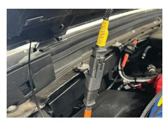
Fig. 18: Connect 3-pin connector to Link Harness.
