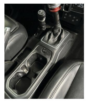
Fig. 32: Reinstall the cup holder/shifter trim.
