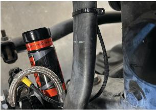
Fig. 24: Zip tie the harness to the sway bar.
