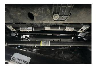
Fig. 22: Route the driver side Link Harness.
