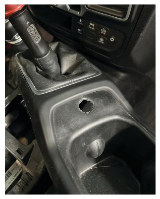
Fig. 5: Drill a hole in the cup holder trim.
