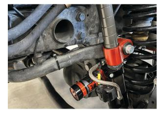
Fig. 25: Connect harness to QSE-Link mating connector.
