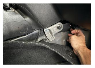
Fig. 11: Lift the carpet to route Controller Harness.
