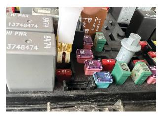
Fig. 27: Remove the yellow fuse from the fuse box.
