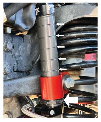
Fig. 2: Grooves (upper small arrows); eyelet nut (lower large arrow).
