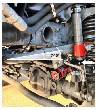
Fig. 1: Installed FOX QSE-Link. Reservoir clamp (arrow).
