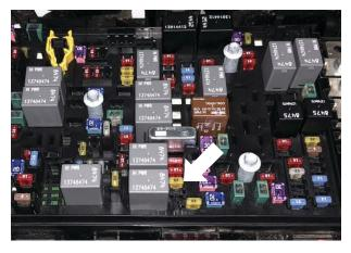
Fig. 26: Remove the yellow fuse from the fuse box.
