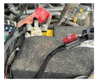
Fig. 29: Install the fuse in the fuse holder.
