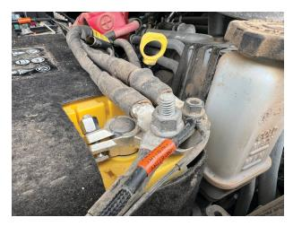
Fig. 31: Connect battery ground cable and GND\_BATTERY ring terminal.
