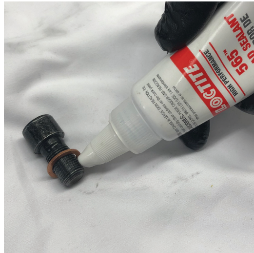
Fig. 27: Apply Loctite to the screw threads.
