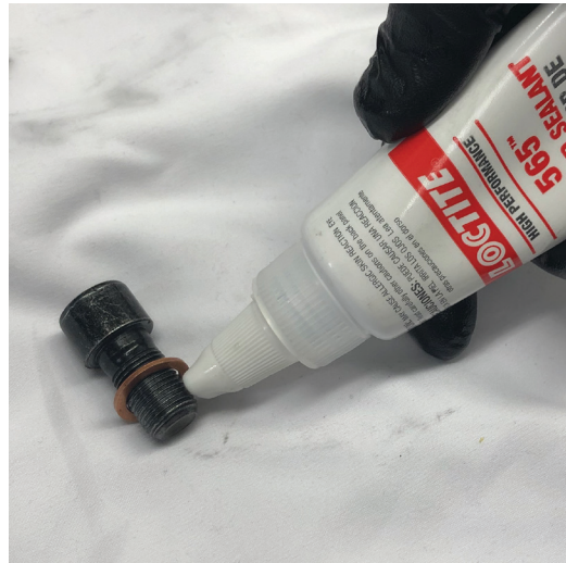
Fig. 13: Apply Loctite to the screw threads.
