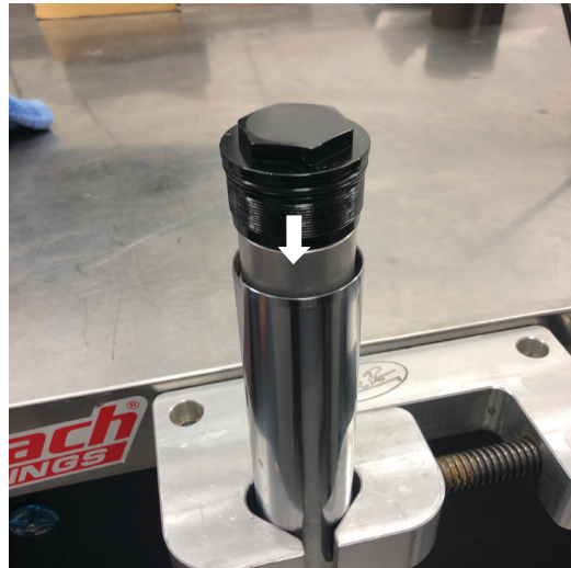
Fig. 24: Carefully clamp the fork leg and compress the assembly.
