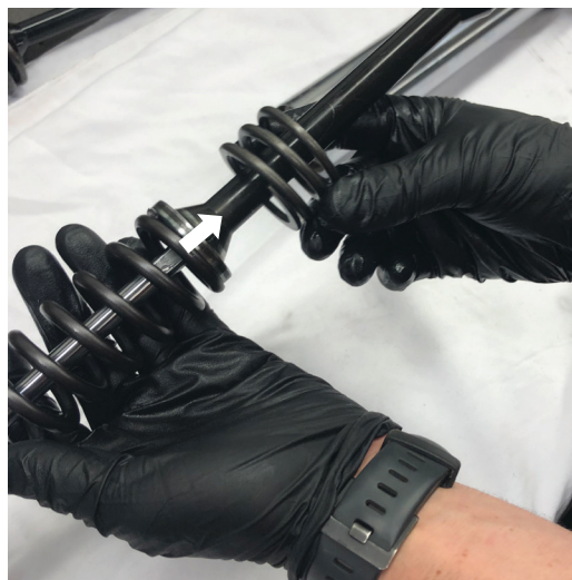
Fig. 22: Install the spring and post.
