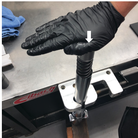
Fig. 31: Compress the cartridge assembly.
