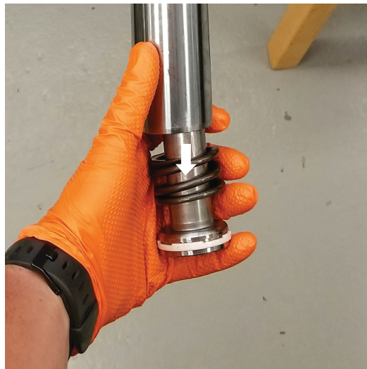
Fig. 9: Remove the damping post and negative spring.
