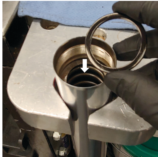
Fig. 16: Install the spring and washer.
