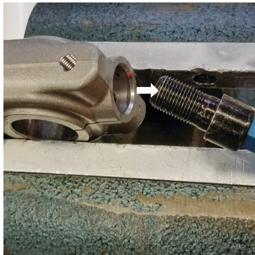
Fig. 8: Remove the retaining screw.
