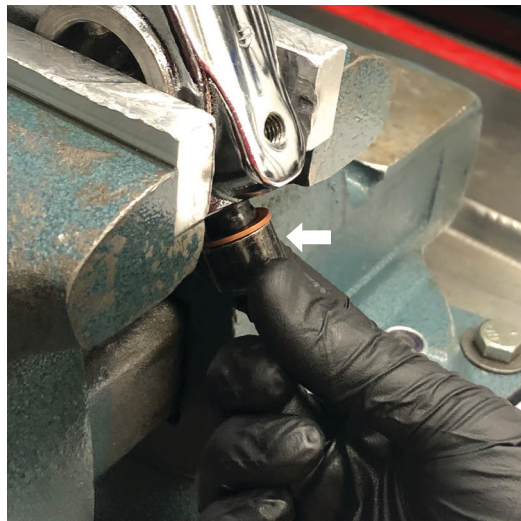
Fig. 28: Install the retaining screw.
