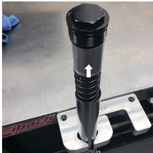
Fig. 29: Slide the lower fork leg up to expose the spring and cartridge.
