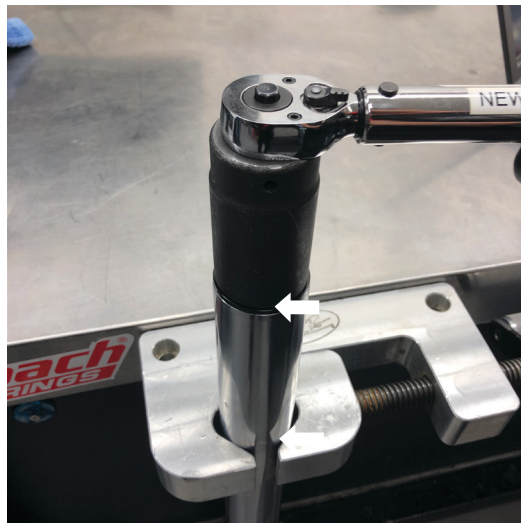
Fig. 32: Torque the top cap.
