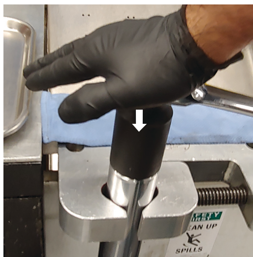
Fig. 2: Downward force while unthreading the top cap.
