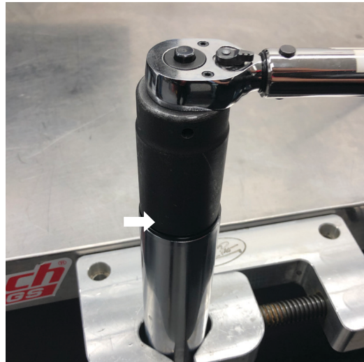
Fig. 20: Torque the top cap.
