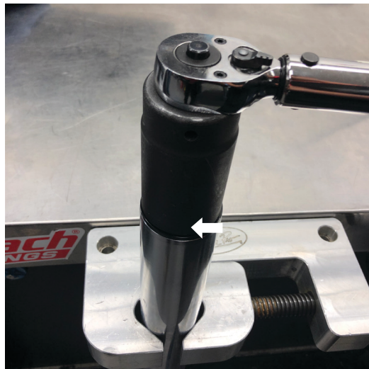
Fig. 25: Thread the top cap.
