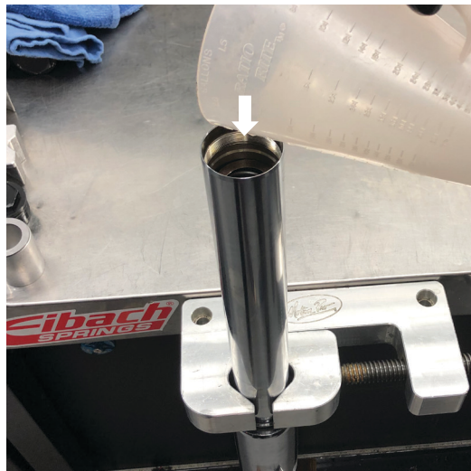
Fig. 17: Add suspension fluid.
