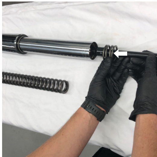
Fig. 11: Install spring and post.
