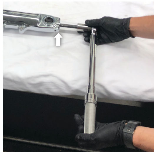
Fig. 15: Install the retaining screw.
