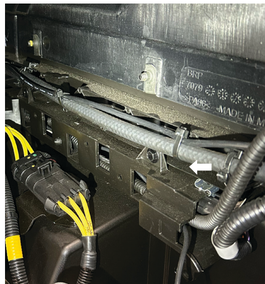
Fig. 13: Zip tie link lead to breather hose.
