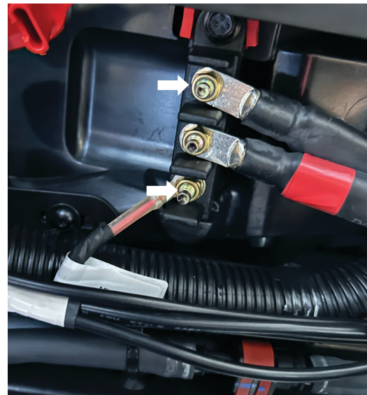
Fig. 10: Install harness adapter onto connector. Black ground wire (upper arrow); orange accessory wire (lower arrow).
