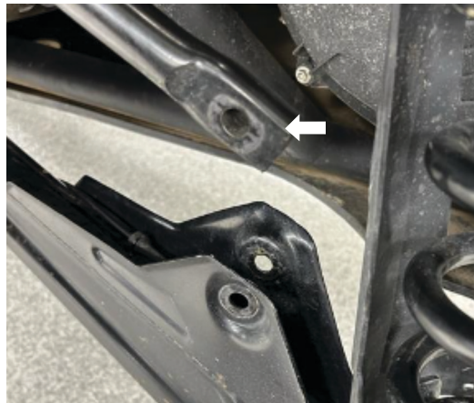
Fig. 2: Remove stock end link.
