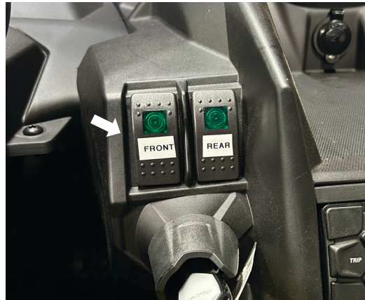
Fig. 5: Remove plugs or cut location for switches.
