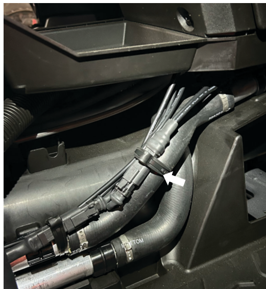
Fig. 7: Zip tie leads to main wiring harness.
