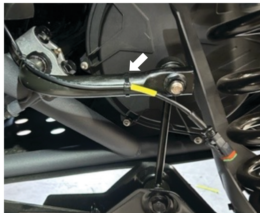
Fig. 16: Zip tie harness to sway bar.
