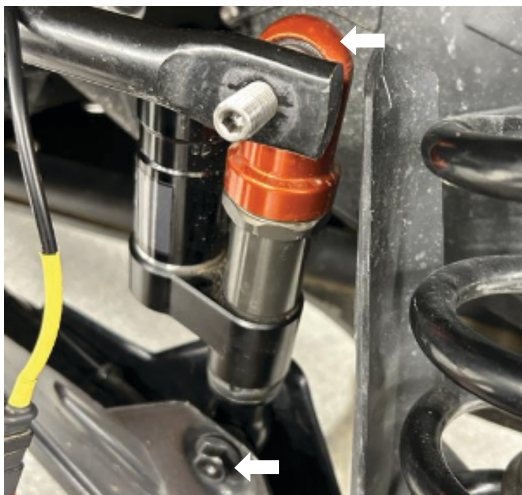
Fig. 3: Tighten the hardware on the new end link.
