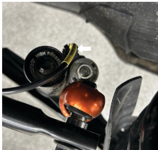
Fig. 4: Plug in the connector.
