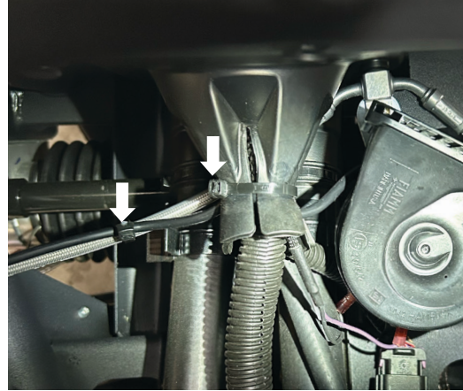
Fig. 8: Zip tie the harness to the brake lines.
