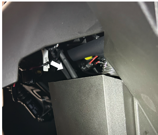
Fig. 6: Route switch harness behind dash.
