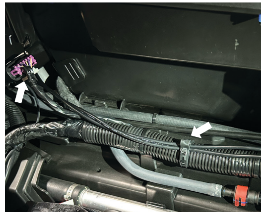
Fig. 12: Zip tie the harness (right arrow). Area for extra length of harness (left arrow).
