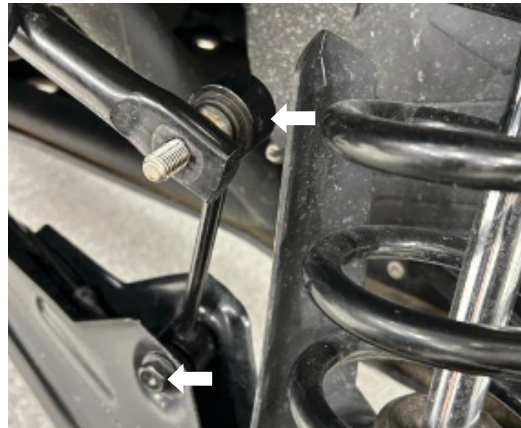
Fig. 1: Remove hardware on stock end link.
