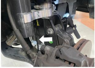
Fig. 19: Route the wire between the strut body and strut hose.
