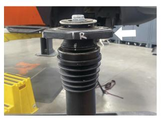
Fig. 12: Remove lower washer from strut boot.
