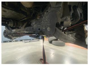
Fig. 4: Secure a ratchet strap on the hub end.
