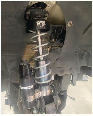
Fig. 16: Loosely install strut onto hub; align tophat with footwell plate.
