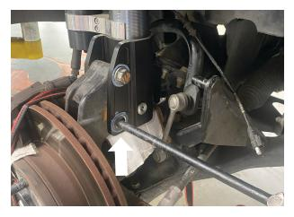
Fig. 5: Insert the bar into lower clevis hole.
