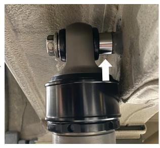
Fig. 22: Thicker reducer toward frame rail.
