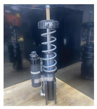
Fig. 14: Remove tophat nut and spacer sleeve.
