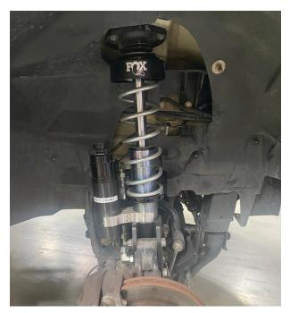
Fig. 20: Final FOX strut installation.
