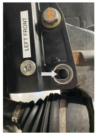
Fig. 17: Position the hub angle to the end of the slot on the lower clevis bolt hole.
