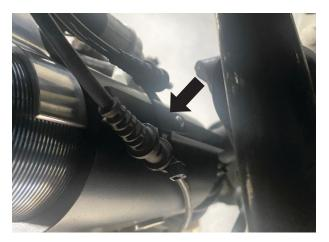
Fig. 18: Secure the brake sensor and ABS wires.
