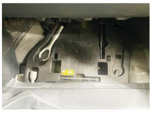
Fig. 7: Unclip the tool tray.
