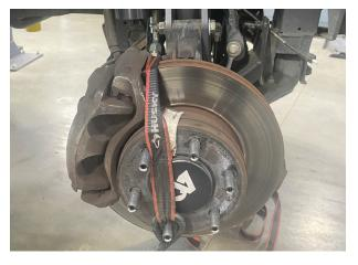
Fig. 3: Secure a ratchet strap on the hub end.
