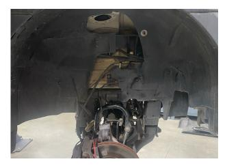
Fig. 11: Remove stabilizing bar from lower clevis hole; remove strut from wheel well.
