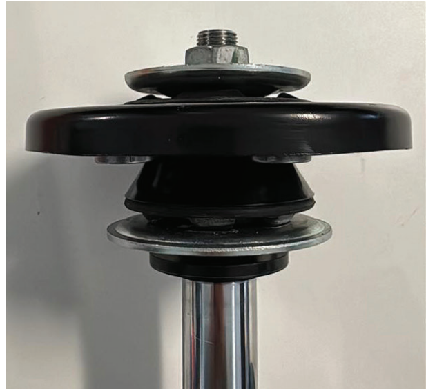
Fig. 17: Install OE tophat components.
