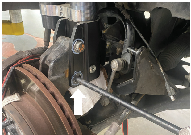
Fig. 5: Insert a bar into lower clevis hole.
