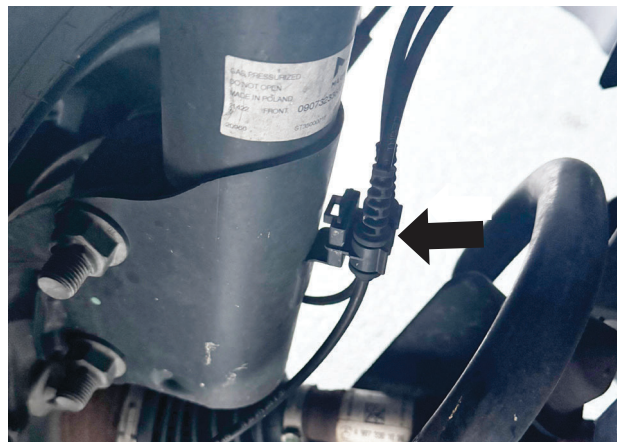
Fig. 1: Unclip the speed sensor and brake sensor wires.
