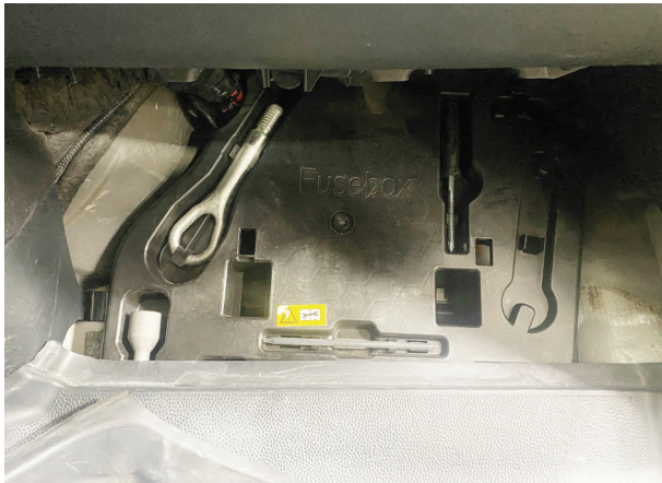
Fig. 7: Unclip the tool tray.
