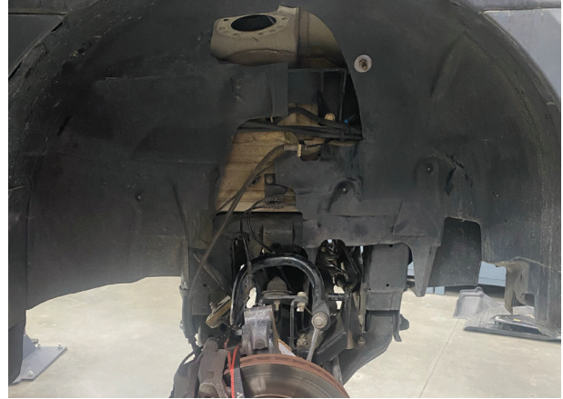
Fig. 11: Remove stabilizing bar from lower clevis hole; remove strut from wheel well.
