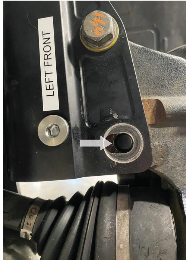
Fig. 20: Position the hub angle to the end of the slot on the lower clevis bolt hole.
