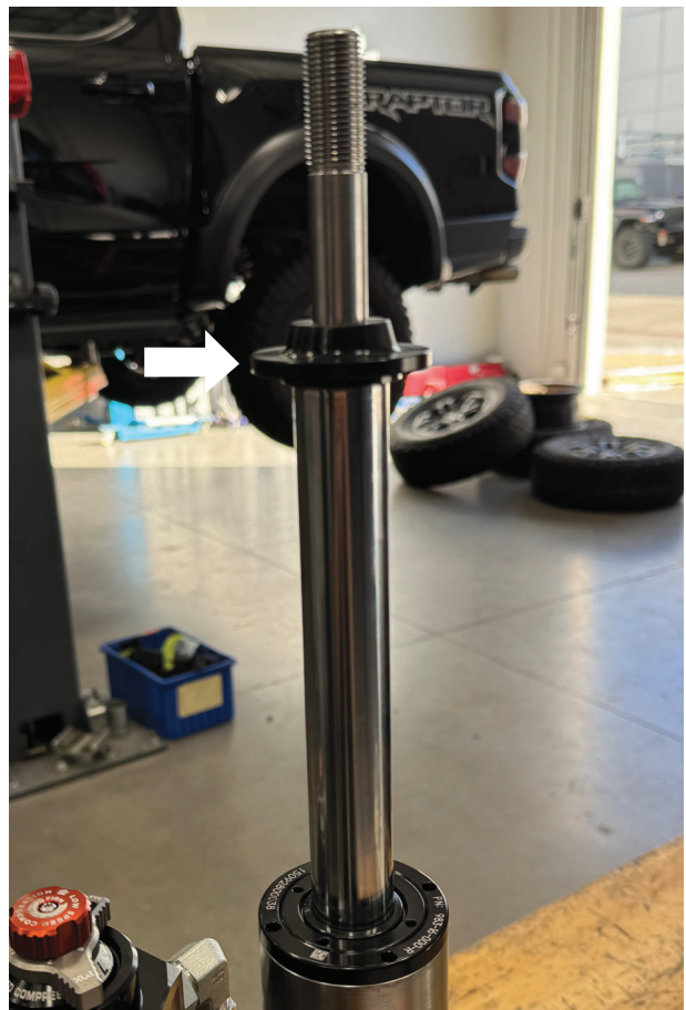
Fig. 16: Install center piece onto shaft.
