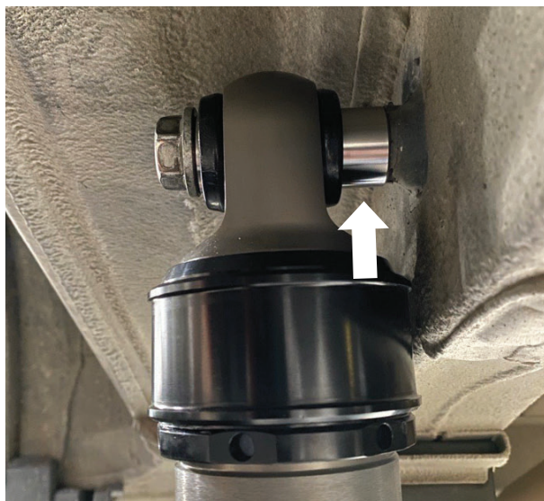
Fig. 26: Thicker reducer toward frame rail.
