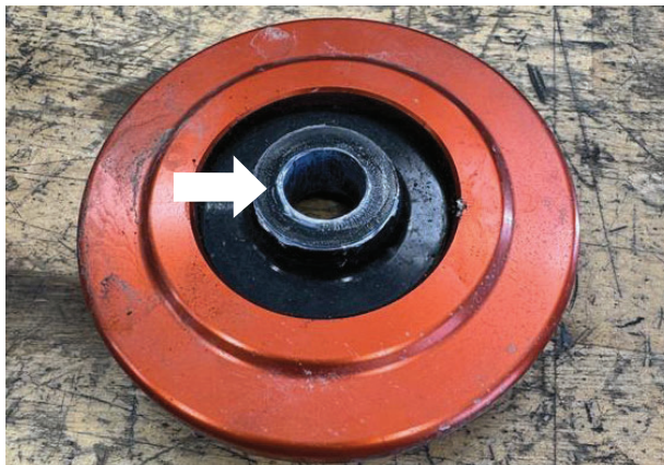
Fig. 15: Remove center piece from provided tophat.
