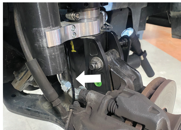
Fig. 22: Route the wire between the strut body and strut hose.
