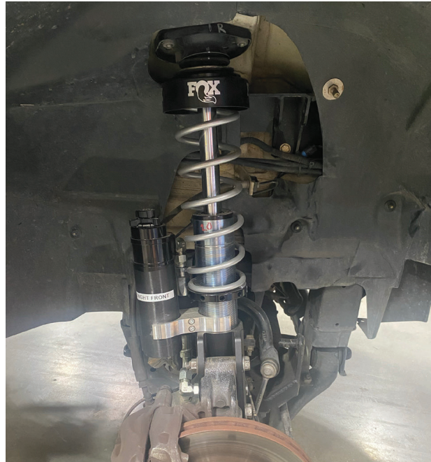
Fig. 23: Final FOX strut installation.
