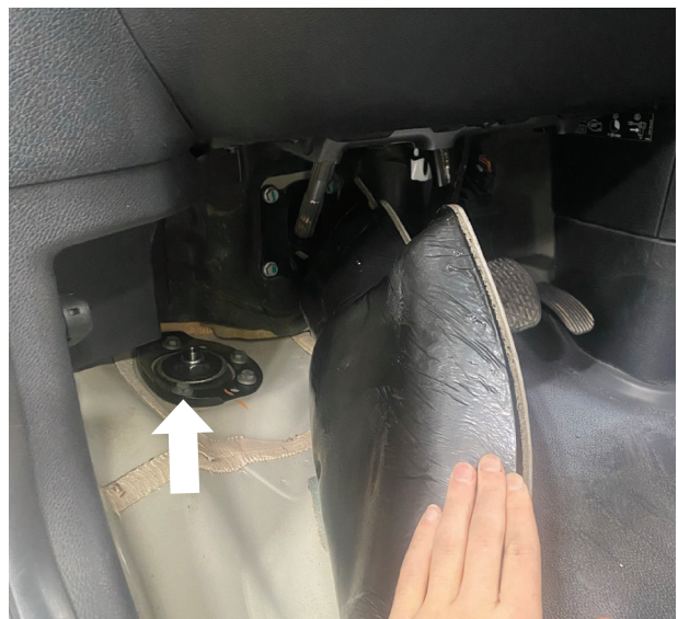
Fig. 10: Lift the footwell floormat to expose tophat bolts.
