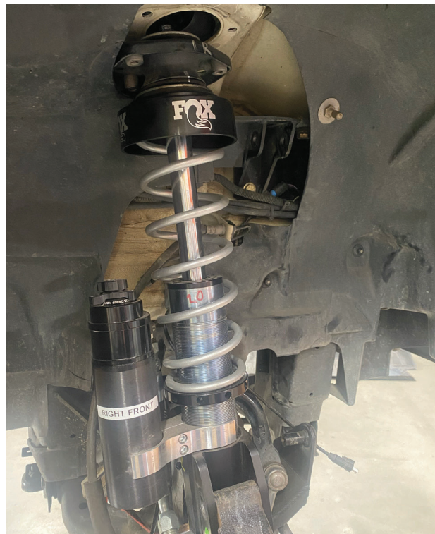
Fig. 19: Loosely install strut onto steering knuckle; align tophat with footwell plate.
