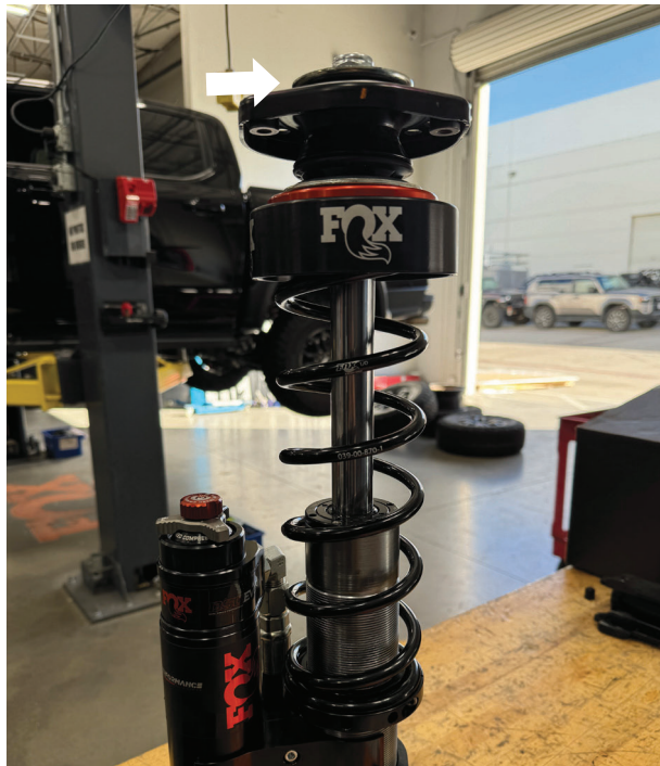
Fig. 18: Install OE tophat components.
