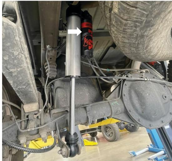
Fig. 4: Reservoir facing center of vehicle (driver side view).
