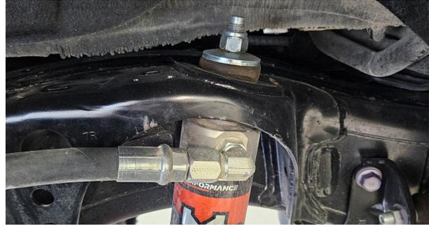
Fig. 21: Install the stem top nut (passenger side shown).
