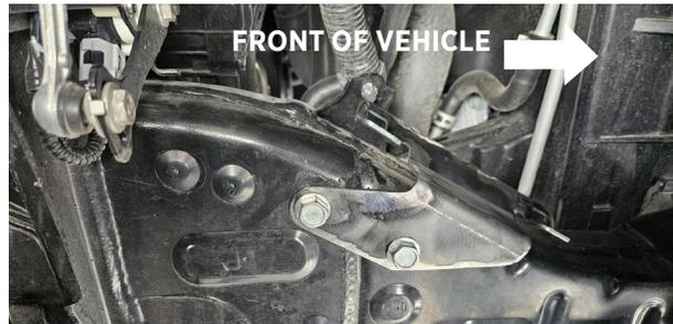
Fig. 5: Install the reservoir bracket assembly.
