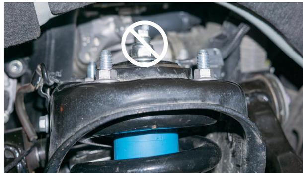
Fig. 7: Remove the four top hat nuts. Do NOT remove the center nut.
