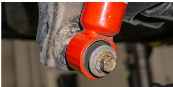
Fig. 18: Remove lower shock mount bolt.
