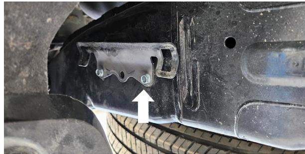
Fig. 20: Install the self tapping screw (passenger side shown).
