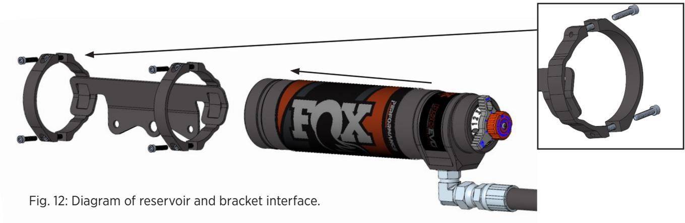
Fig. 12: Diagram of reservoir and bracket interface.
