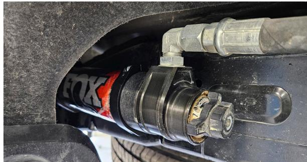
Fig. 23: Mount the reservoir to the bracket (driver side shown).
