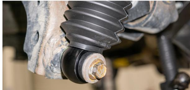
Fig. 22: Install the lower shock bolt (passenger side shown).
