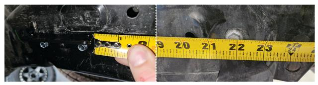
Fig. 19: Drill two pilot holes.
