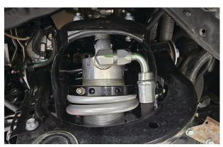
Fig. 9: The hose fitting faces outboard.
