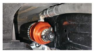
Fig. 23: Mount the reservoir to the bracket (driver side shown).
