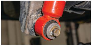
Fig. 18: Remove lower shock mount bolt.
