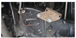
Fig. 5: Fasten the bracket.
