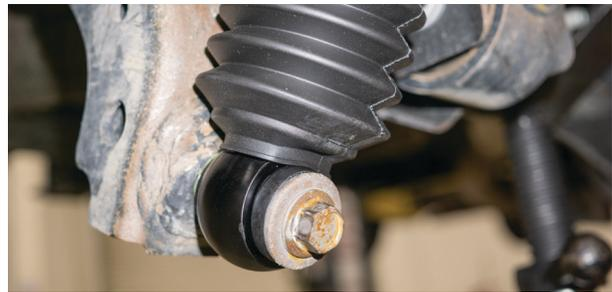
Fig. 21: Install the lower shock bolt (passenger side shown).
