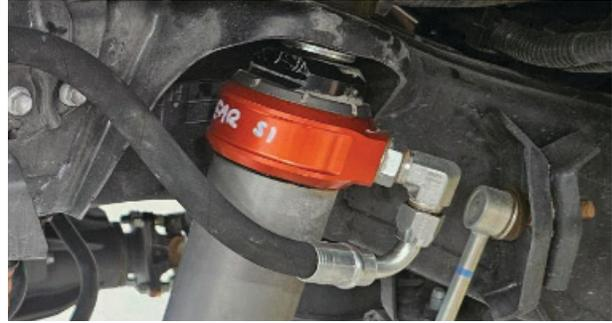
Fig. 20: Install the stem top nut (passenger side shown).
