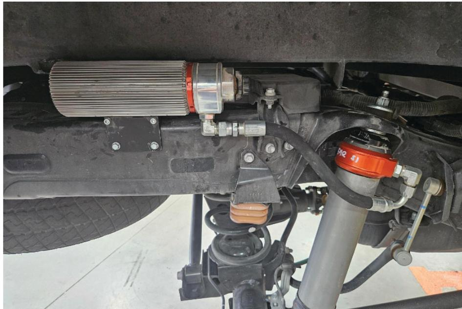
Fig. 22: Mount the reservoir to the bracket (passenger side shown).
