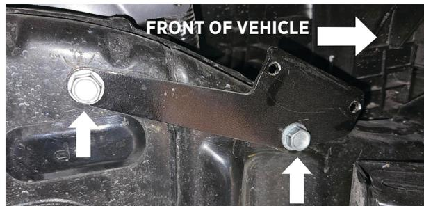
Fig. 5: Install the reservoir bracket assembly.
