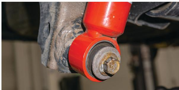
Fig. 18: Remove lower shock mount bolt.
