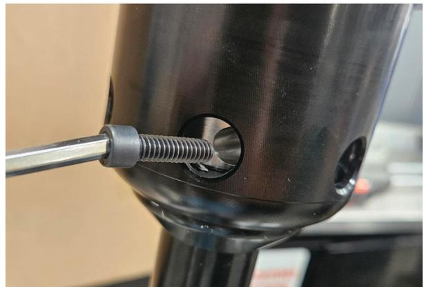
Fig. 16: Screws to clamp spacers to shaft.
