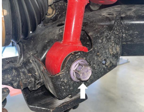
Fig. 7: Remove the bolt from the lower control arm.
