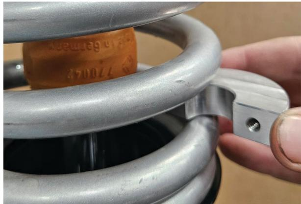
Fig. 15: Slide spacers through spring.
