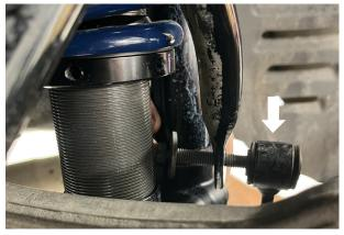
Fig. 22: Reconnect the link using stock hardware on both sides of the vehicle.
