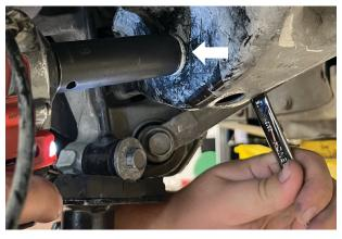
Fig. 16: Remove the lower shock bolt.
