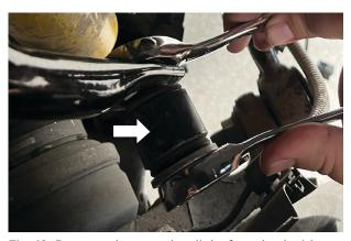
Fig. 12: Remove the sway bar links from both sides.
