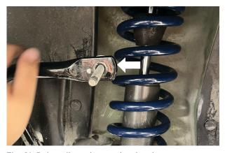
Fig. 21: Reinstall stock sway bar hardware.
