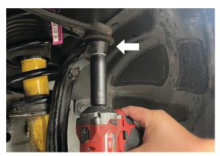
Fig. 7: Remove the upper ball joint.
