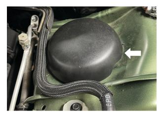
Fig. 4: Remove the black cap.
