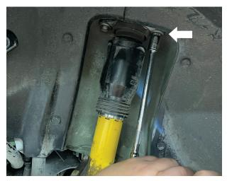
Fig. 15: Remove the upper shock bolts.
