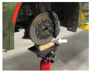
Fig. 6: Support the suspension.
