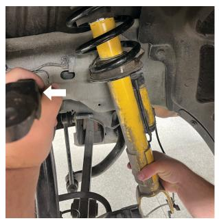
Fig. 8: Hold the spindle, remove the shock.
