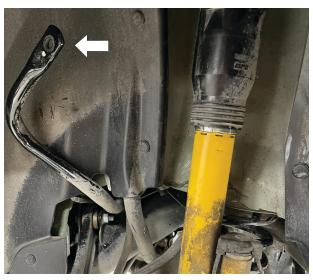
Fig. 13: Swing the sway bar out of the way, remove the stock bolt.
