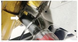
Fig. 2: Remove the sway bar nuts.
