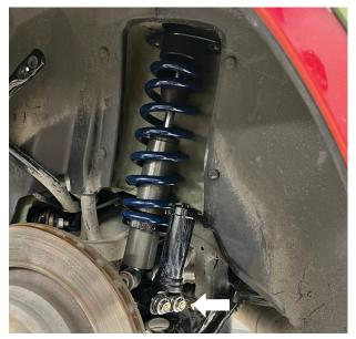
Fig. 20: Install the new shock assembly, adjusters facing outward.
