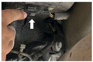
Fig. 11: Remove the clips for vehicles with adaptive damping system.
