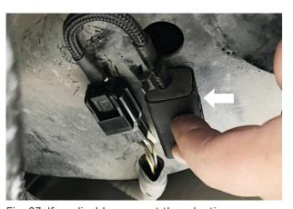
Fig. 23: If applicable, connect the adaptive damping system connector.
