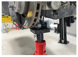
Fig. 14: Support the suspension toward the outside of lower control arm.
