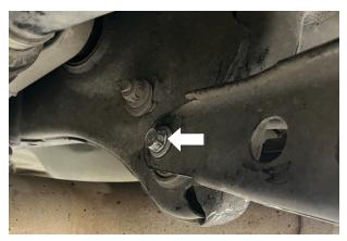
Fig. 19: Align lower control arm to chassis, reinstall hardware.
