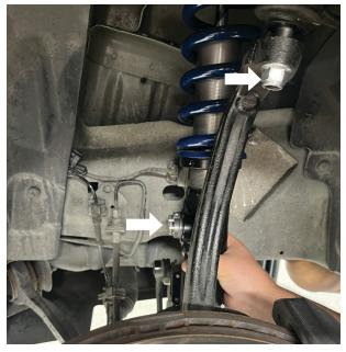
Fig. 9: Install shock with adjusters facing forward; loosely install ball joint nut.
