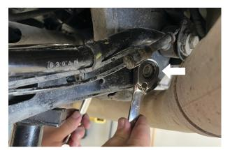
Fig. 18: Remove the inner lower control arm bolt.
