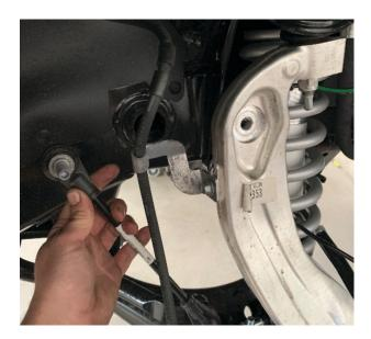
Fig. 1: Disconnect sway bar from spindle.
