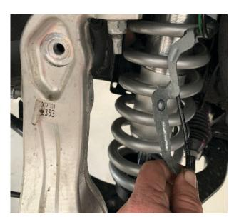
Fig. 3: Disconnect ABS bracket (passenger side shown).
