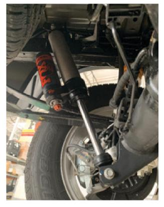
Fig. 10: Install the shock hardware (driver side shown).
