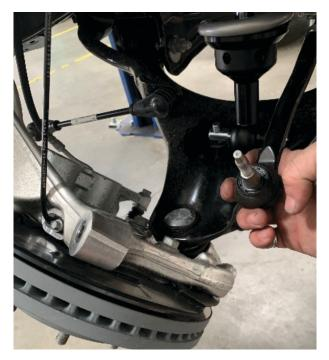
Fig. 5: Disconnect the outer tie rod end (passenger side shown).
