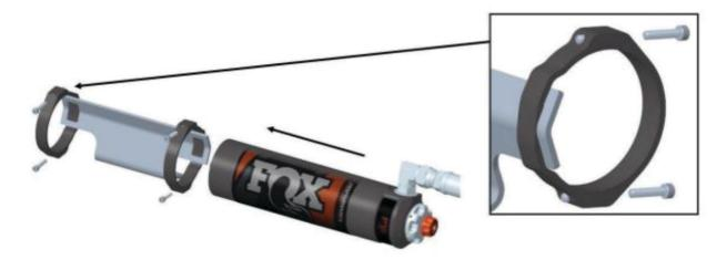
Fig. 9: Diagram of reservoir and clamps.
