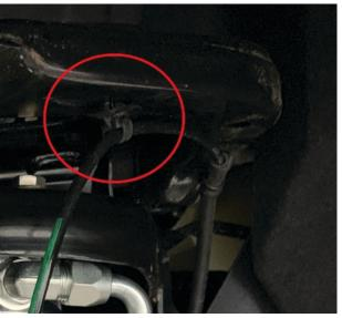
Fig. 4: Disconnect ABS wire clip (passenger side shown).
