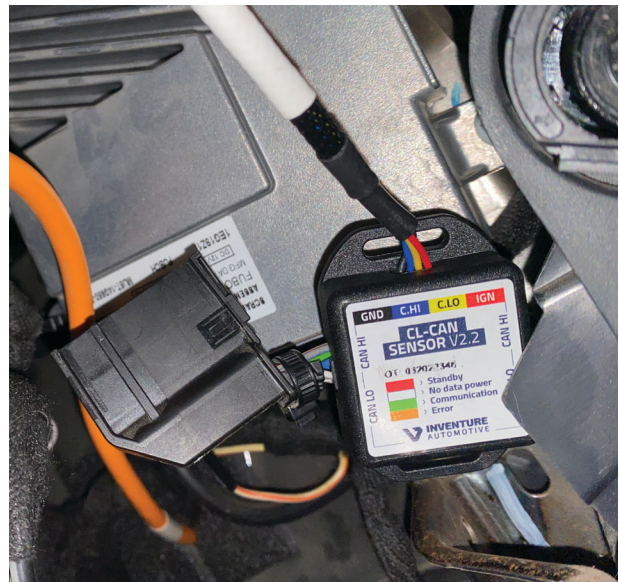
Fig. 43: Install blue and white wire on the CAN reader. Fig. 44: Reattach the back of the CAN reader.
