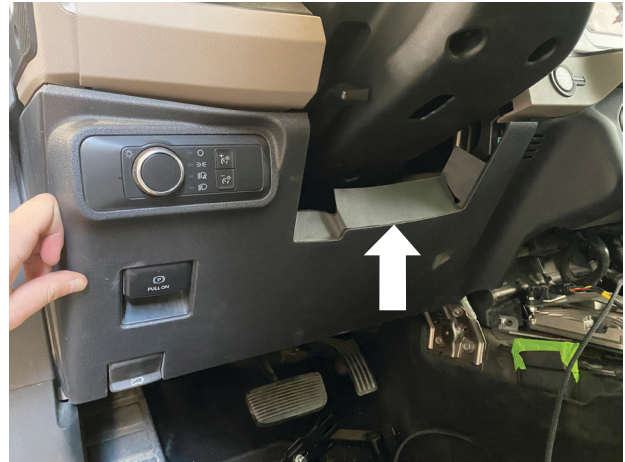
Fig. 36: Pull on the lower panel.
