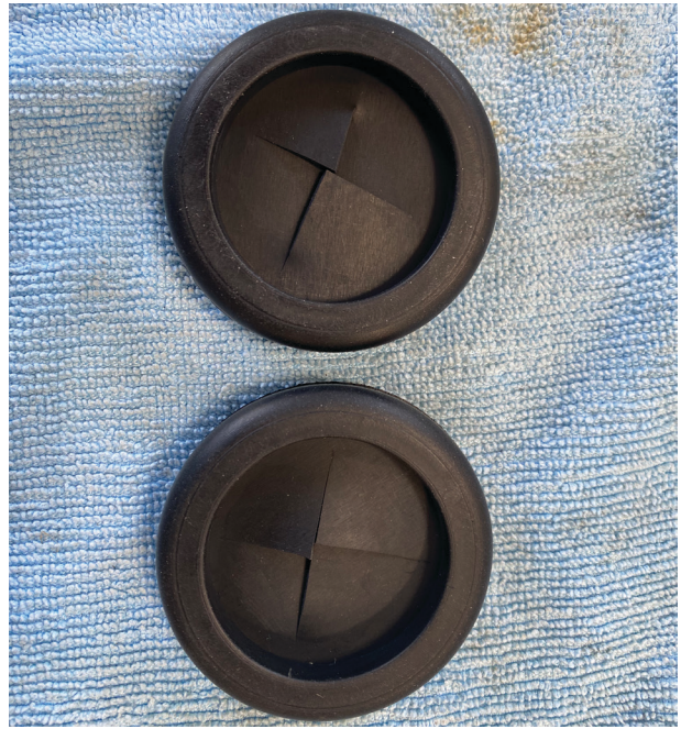
Fig. 29: Cut an "X" pattern into the grommets.
