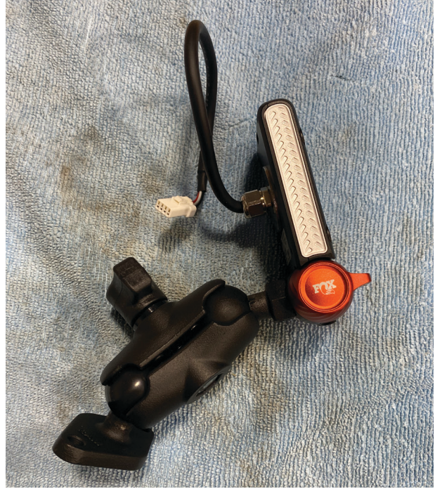
Fig. 28a: Ball mount and touchpoint assembly.
