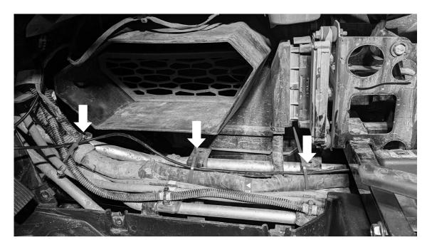
Fig. 38: Loosely secure the rear harness.
