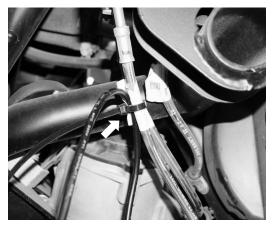
Fig. 24: Wire cable tied to brake line below reservoir.
