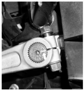
Fig. 3: Mark the spline and arm orientation.
