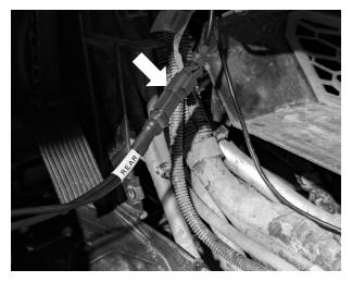
Fig. 37: Connect rear harness to rear QSE link.
