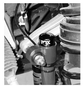
Fig. 19: Wire routing above upper control arm.
