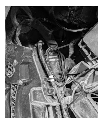
Fig. 41: Secure excess wire to main harness.
