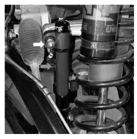
Fig. 6: Tighten the hardware on the upper end link (white arrow). Reservoir faces inward (orange arrow).
