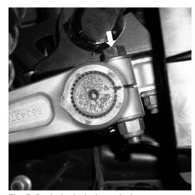
Fig. 5: Push the bolt through the arm.
