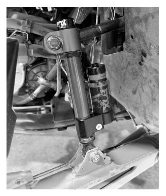
Fig. 26: Install the FOX QSE-Link and the lower link mount OE hardware.
