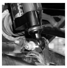
Fig. 7: Tighten the hardware on the lower end link.
