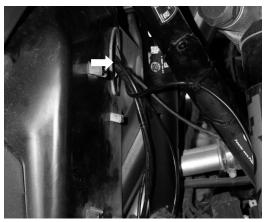
Fig. 16: Route wiring through grommet hole.
