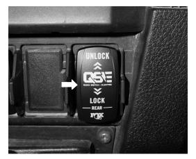
Fig. 15: Push the switch into the dash.
