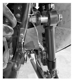
Fig. 40: Loosely zip tie harness to sway bar and QSE Link.
