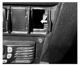
Fig. 11: Remove accessory switch cover.
