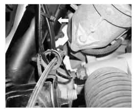
Fig. 21: Wire routing above upper control arm.
