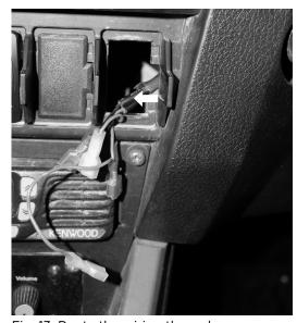
Fig. 13: Route the wiring through accessory switch.
