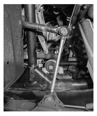
Fig. 25: Remove the stock end link.
