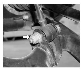
Fig. 1: Remove stock end link.
