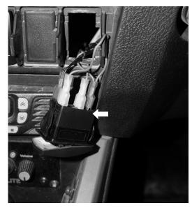
Fig. 14: Plug the switch into the wiring.
