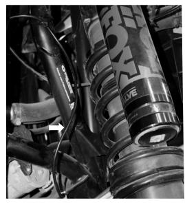
Fig. 18: Clearance during suspension movement.
