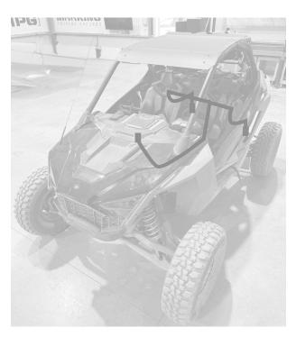
Fig. 27: Rear harness kit routing.
