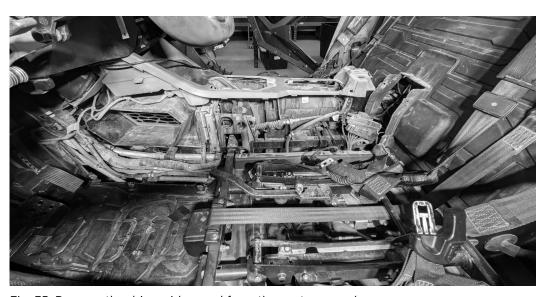
Fig. 35: Remove the driver side panel from the center console.
