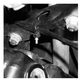
Fig. 22: Wire cable tied to bulkhead.
