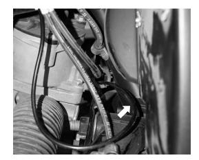
Fig. 23: Wire routing through driver side loop.
