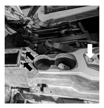
Fig. 32: Remove center bolt (white arrow). Disengage quick release knobs (black arrows).
