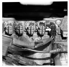
Fig. 10: Install the FOX 3-pin connector.
