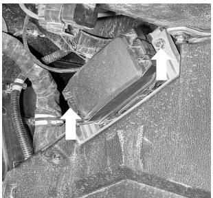
Fig. 31: Remove fuse box bolts.
