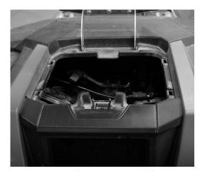
Fig. 9: Remove the center console liner.
