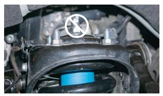
Fig. 4: Remove the four top hat nuts. Do NOT remove the center nut.
