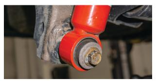
Fig. 11: Remove lower shock mount bolt.
