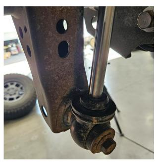
Fig. 13: Install the lower shock bolt (passenger side shown).
