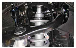
Fig. 6b: The side without the nitrogen port faces outboard (2.5).
