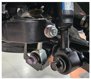
Fig. 9b: Sway bar end link (with KDSS).
