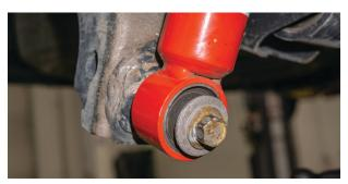
Fig. 11: Remove lower shock mount bolt.
