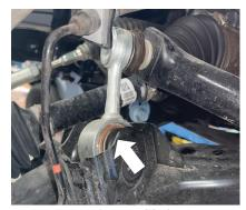
Fig. 2a: Sway bar end link (non-KDSS).
