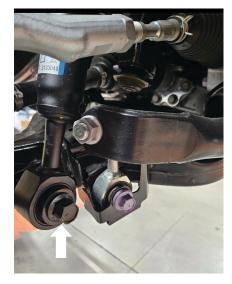
Fig. 5: Remove the bolt from the lower control arm.
