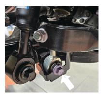
Fig. 2b: Sway bar end link (with KDSS).
