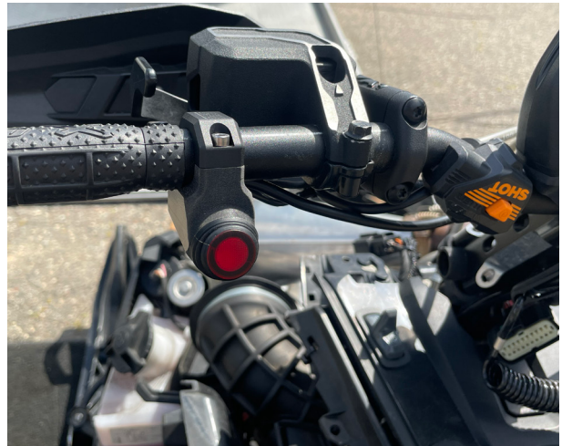
Fig. 18: Switch lead routing
