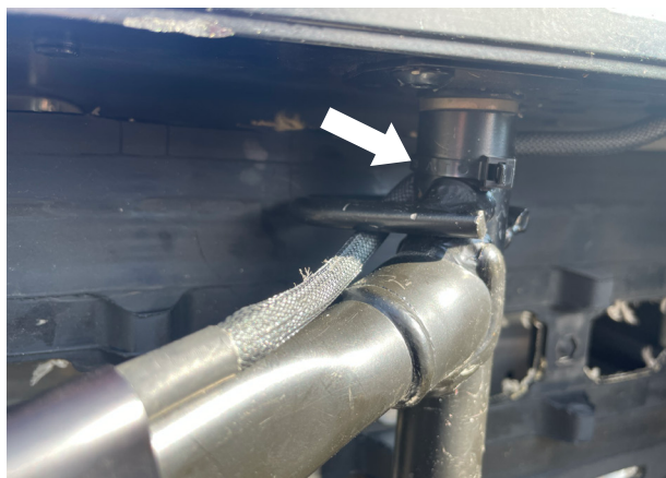
Fig. 10: Secure the wire harness onto the front pivot tube with a cable tie.
