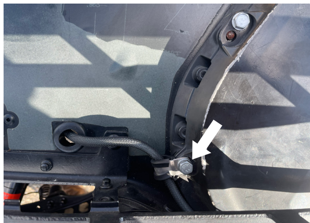
Fig. 11: Secure the harness routing clip.
