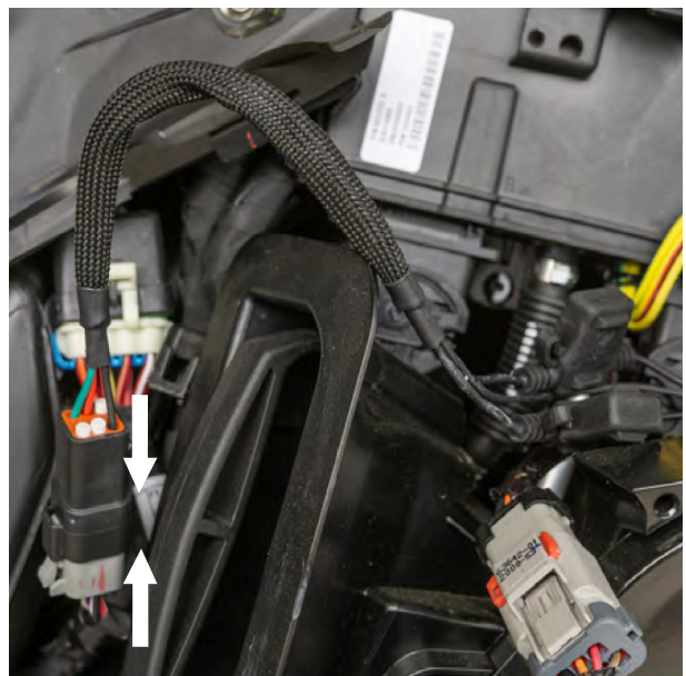
Fig. 13: Plug the accessory plug into the QSE mating power connector.
