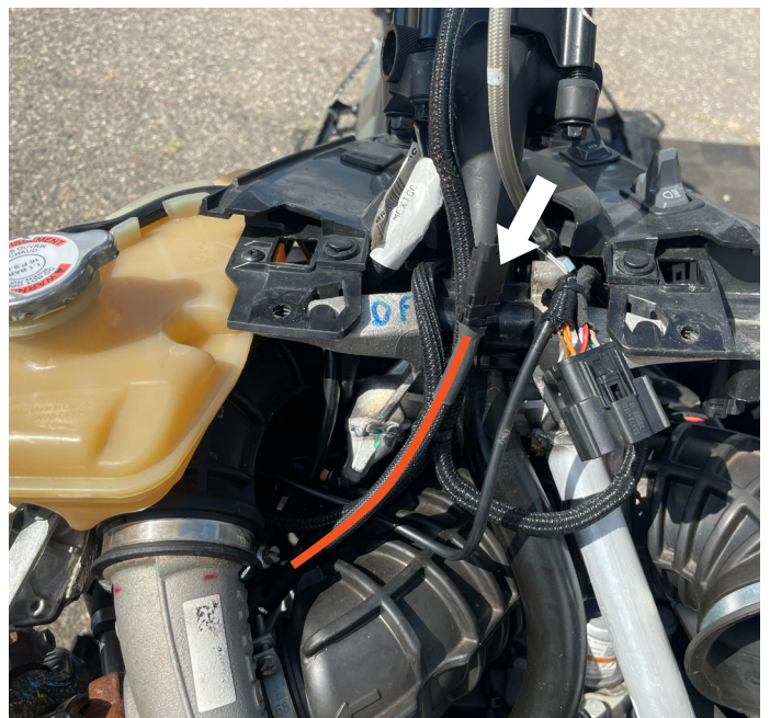
Fig. 16: Route the switch lead (red line); plug into switch harness in a later step (arrow)
