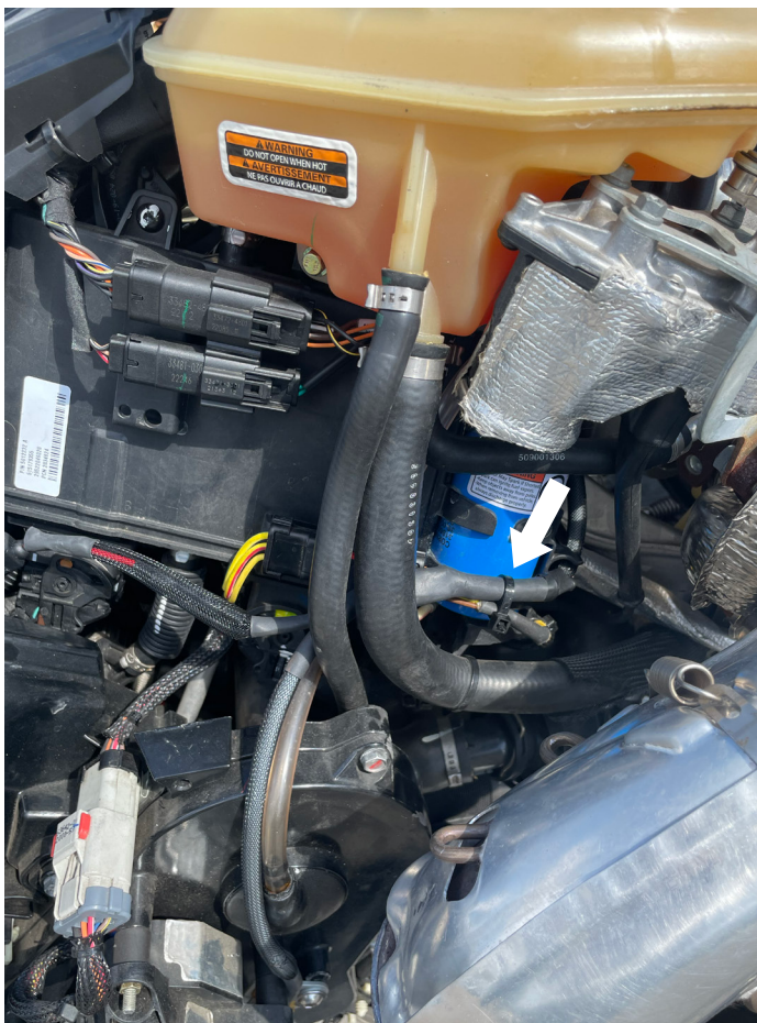
Fig. 15: Secure the main harness to the vehicle harness
