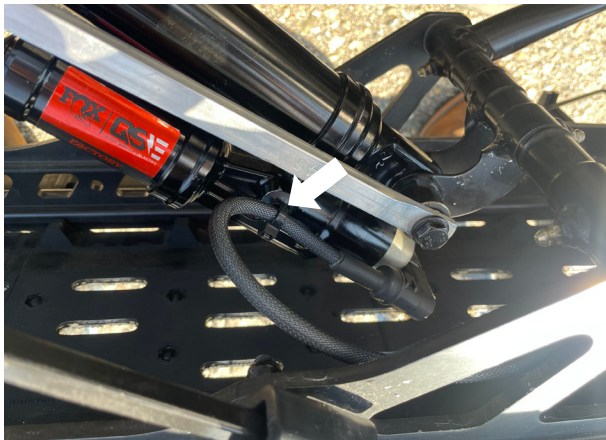
Fig. 6: Plug the track harness into the rear track shock. Install the routing clip as shown.
