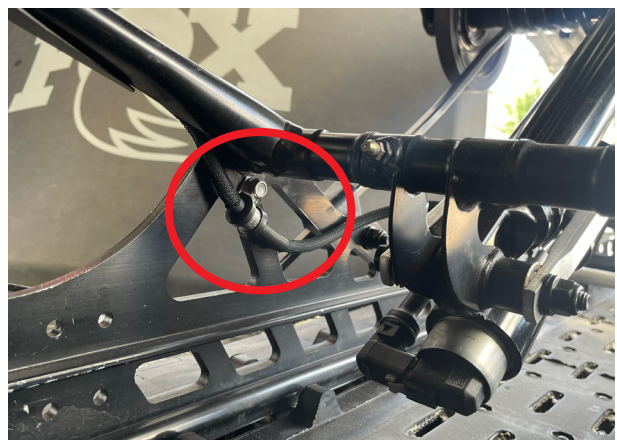
Fig. 7: Secure the track harness to the inside of the right hand rail, using the hole from Fig. 5.
