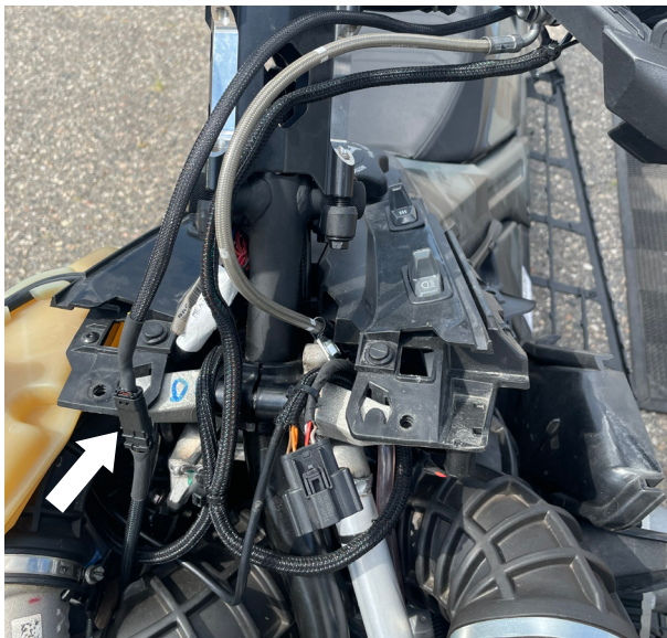
Fig. 19: Switch lead routing
