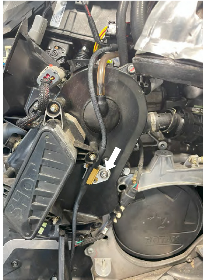
Fig. 14: Main harness routing and resistor orientation
