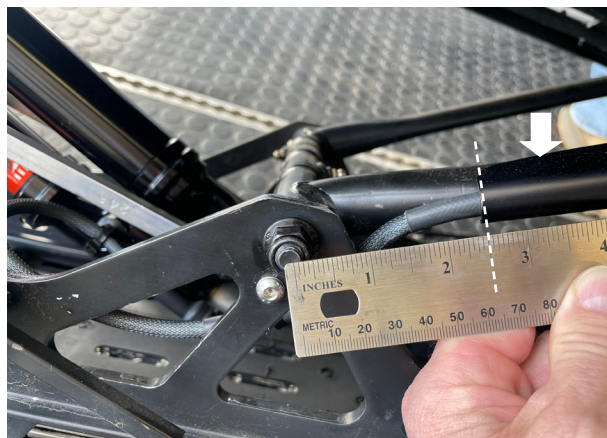
Fig. 8: Place the guard along the front torque arm, center the heat shrink on the edges of the guard.
