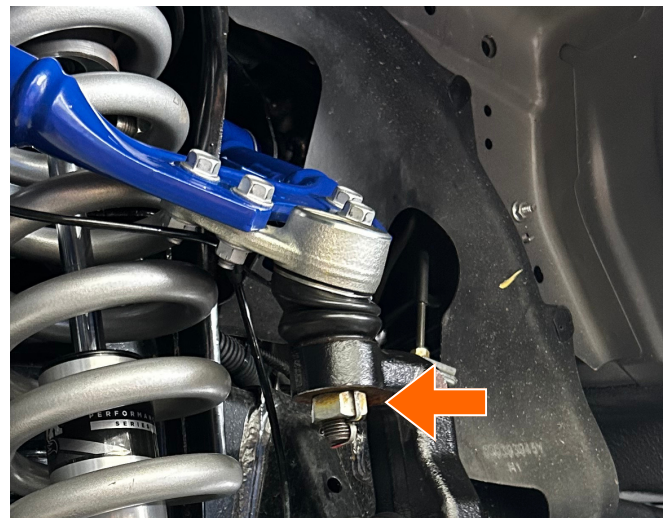
Fig 9: Reattach the UCA to the upright.
