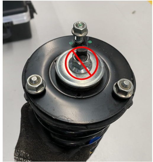
Fig. 4: Remove the three top hat nuts. Do NOT remove the center nut.
