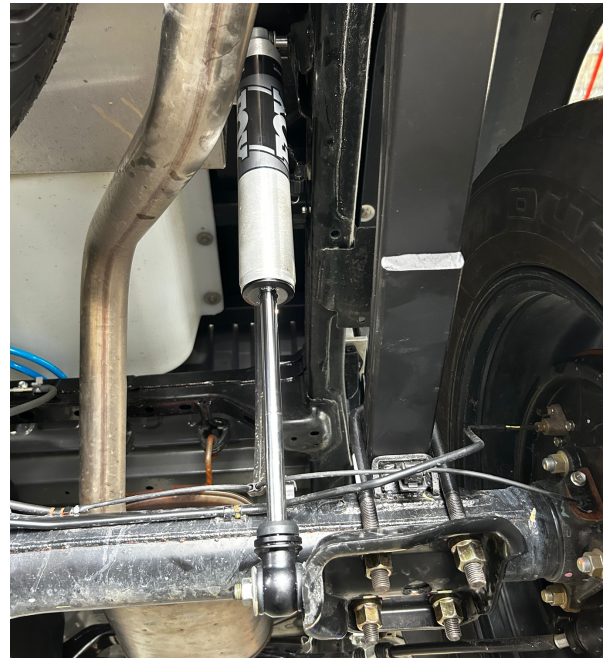
Fig 13: Rear FOX shock installed
