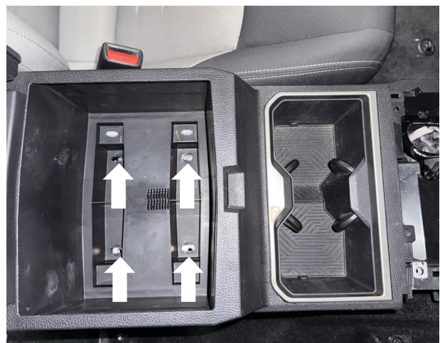
Fig. 44: Confirm bolt alignment in center console storage area.
