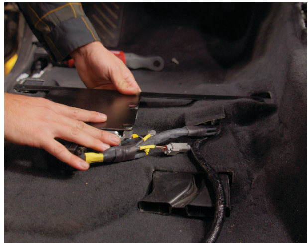
Fig. 40: Place ECU at the driver seat area.
