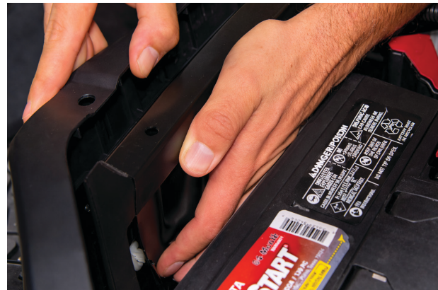
Fig. 71: Push forward to release clips.
