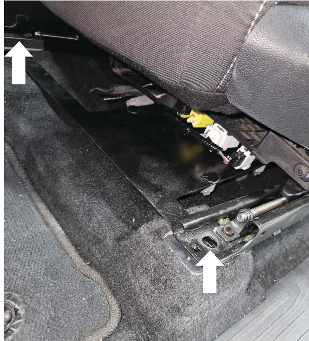
Fig. 85: Install the ECU bracket onto the rails.
