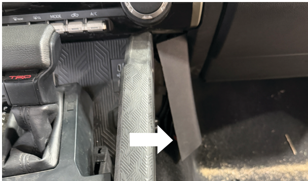
Fig. 11: Pull the trim toward the passenger door.
