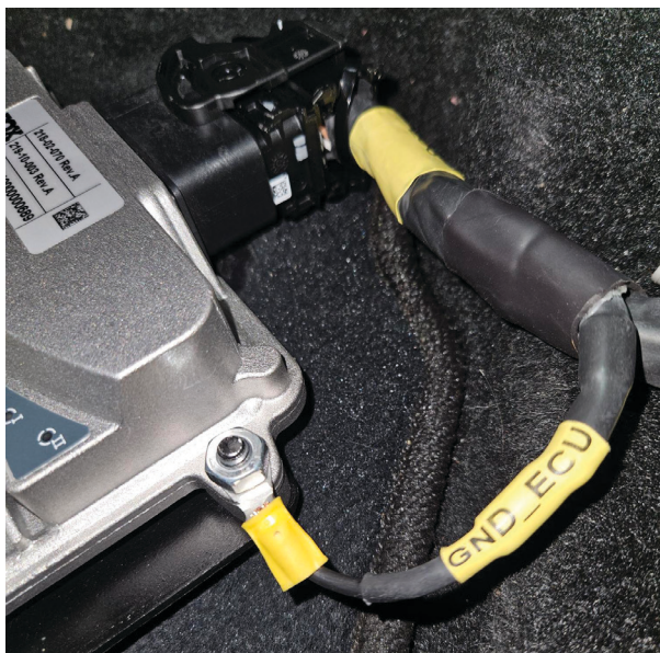
Fig. 39: GND_ECU and 4th nut assembled.
