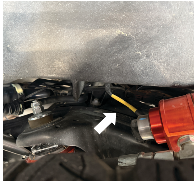
Fig. 61: Plug RLC connector into shock.
