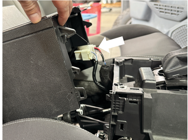
Fig. 15: Disconnect white connectors.
