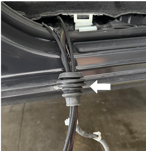
Fig. 49: Install OE ground harness into FOX grommet/wiring assembly.
