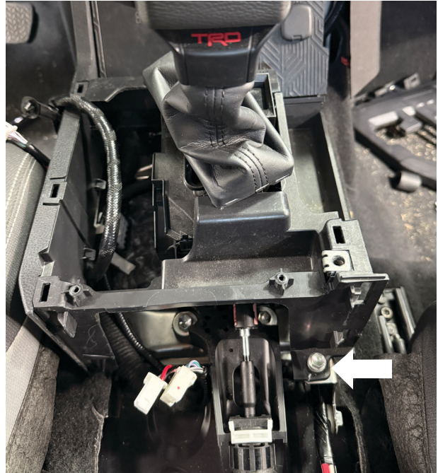
Fig. 19: Remove bolt under center console.
