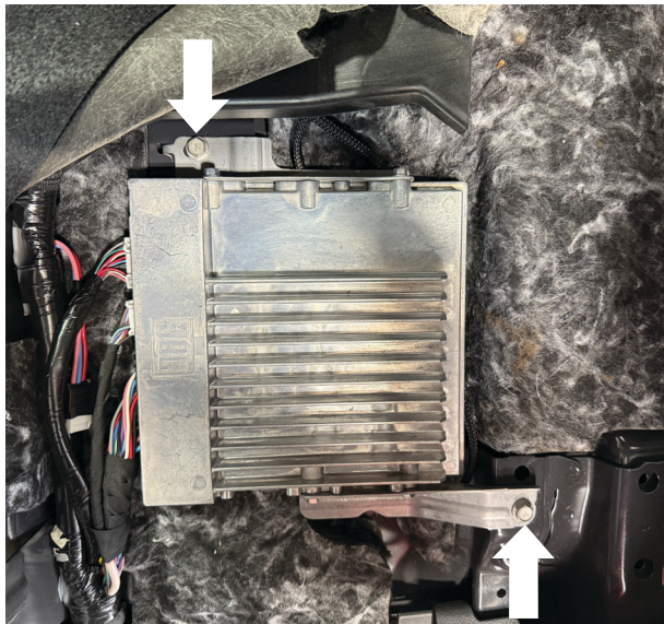
Fig. 52: Remove bolts on OE bracket/module.
