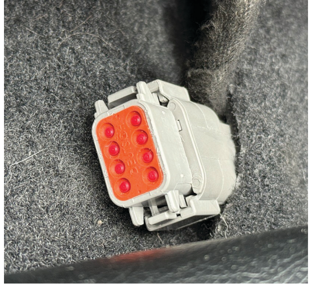
Fig. 54: Install 8-pin dust cap.
