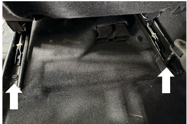
Fig. 27: Remove rear bolts.
