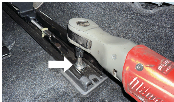
Fig. 28: Remove rear bolts.
