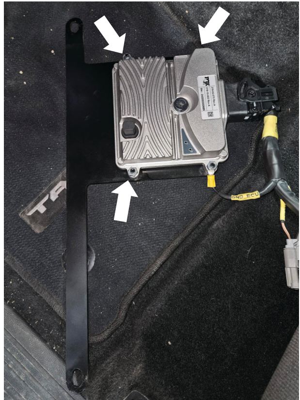
Fig. 38: Align the ECU/PEM studs on the bracket; 3 nuts assembled first.
