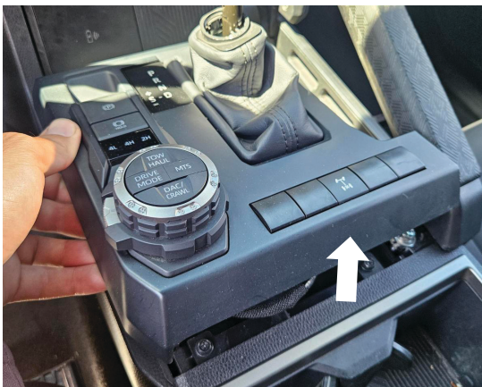
Fig. 4: Lift the shifter trim over the lever.
