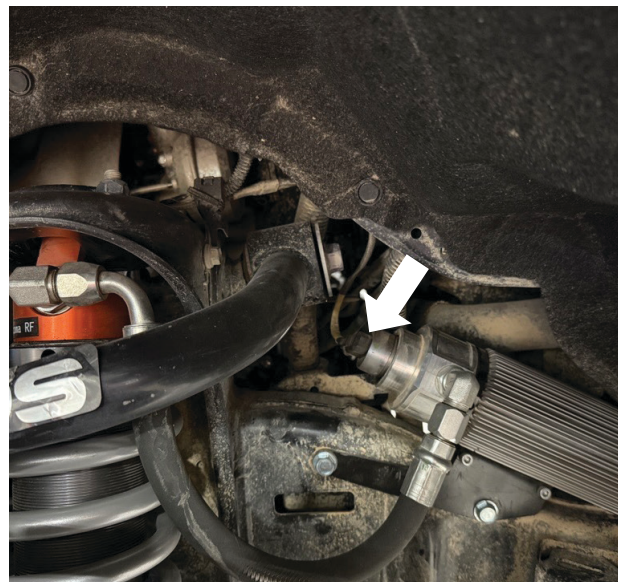
Fig. 64: Plug FRC connector into shock.
