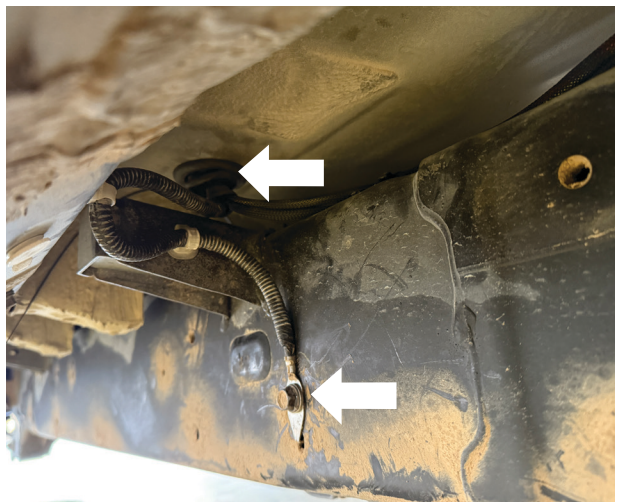
Fig. 50: Route wires into hole; install the FOX grommet (top arrow); reattach OE ground cable bolt (bottom arrow).
