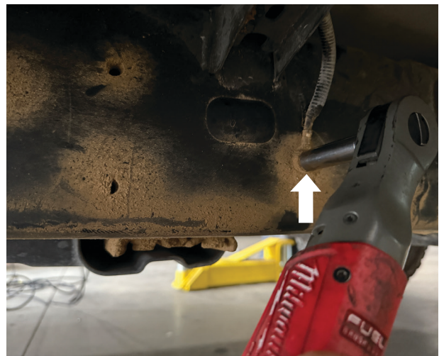
Fig. 47: Remove the OE ground cable bolt.
