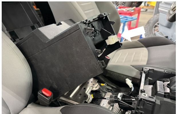
Fig. 16: Disconnected white connectors.
