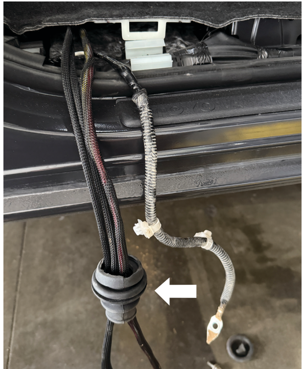
Fig. 48: Remove the OE grommet, pull wiring into cab.
