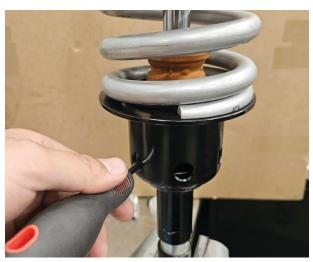
Fig. 24: Lift the bump stop with a screwdriver.
