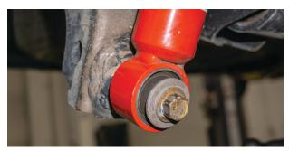
Fig. 29: Remove lower shock mount bolt.
