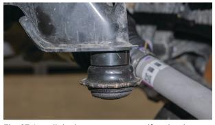
Fig. 27: Install the bump stop spacer if preload is added.
