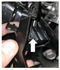
Fig. 11c: Lift the tab to remove the connector
