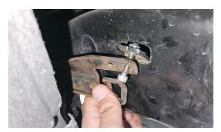
Fig. 32: Insert the nut plate
