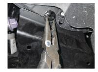
Fig. 5: Remove the splash guard
