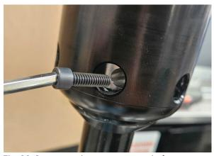
Fig. 26: Screws to clamp spacers to shaft.
