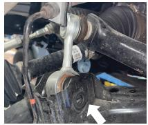
Fig. 2b: Sway bar end link (non-KDSS)
