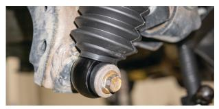
Fig. 36: Install the lower shock bolt (passenger side shown).
