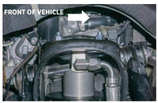
Fig. 16: The hose fitting faces outboard.
