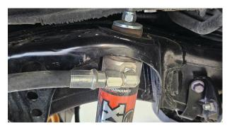
Fig. 35: Install the stem top nut (passenger side shown).
