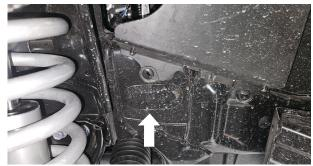
Fig. 4: Remove the plastic plugs.
