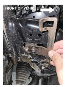
Fig. 7: Place the nut plate into the hole
