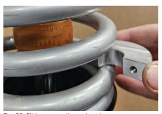
Fig. 25: Slide spacers through spring.
