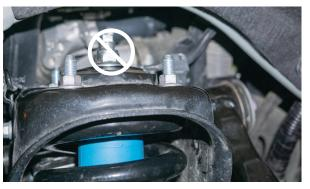
Fig. 14: Remove the four top hat nuts. Do NOT remove the center nut.
