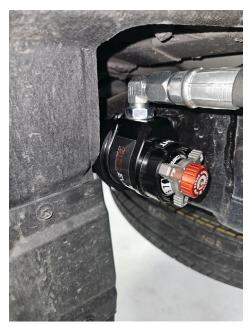
Fig. 37: Mount the reservoir to the bracket (passenger side shown).
