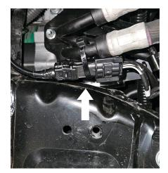
Fig. 12: Zip tie the connector to the lower KDSS hose
