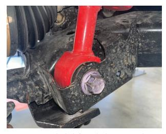
Fig. 15: Remove the bolt from the lower control arm.
