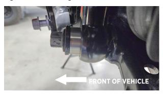
Fig. 17: The large reducer faces forward
