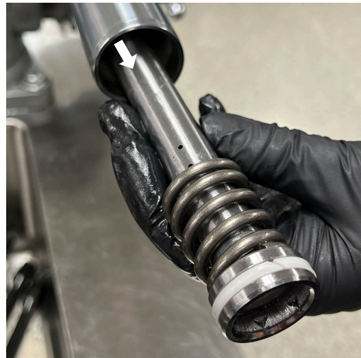
Fig. 7: Remove the damping post and negative spring.
