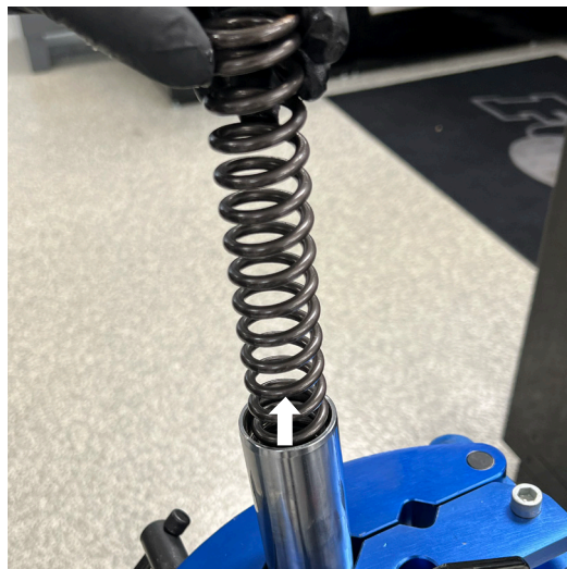
Fig. 5: Remove the spring.
