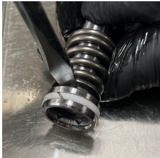
Fig. 8: Pry the damping post and negative spring, if needed.
