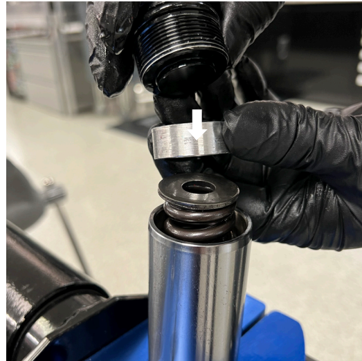
Fig. 17: Install preload spacer and spring washer.
