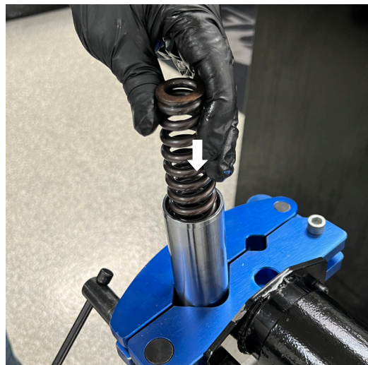
Fig. 15: Install the spring.
