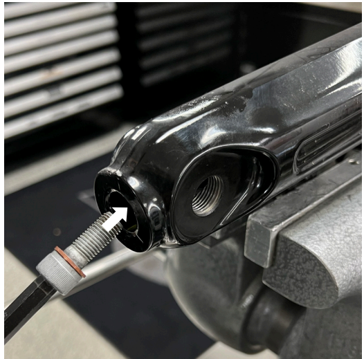
Fig. 23: Install the retaining screw.
