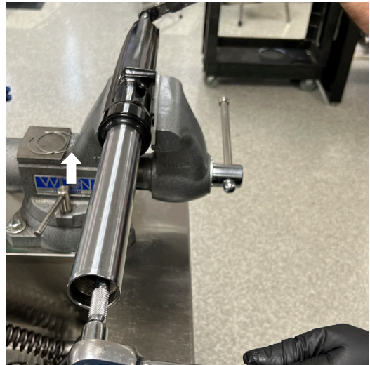
Fig. 14: Hold the extender post. Install the retaining screw
