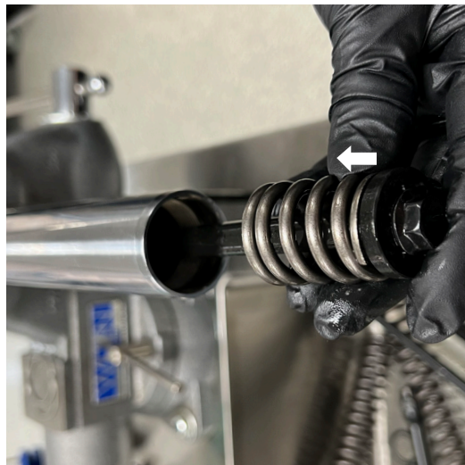
Fig. 10: Install spring and post.
