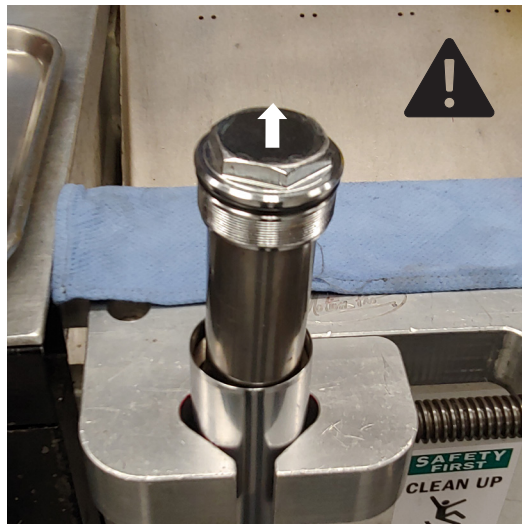
Fig. 2: Carefully remove the top cap.
