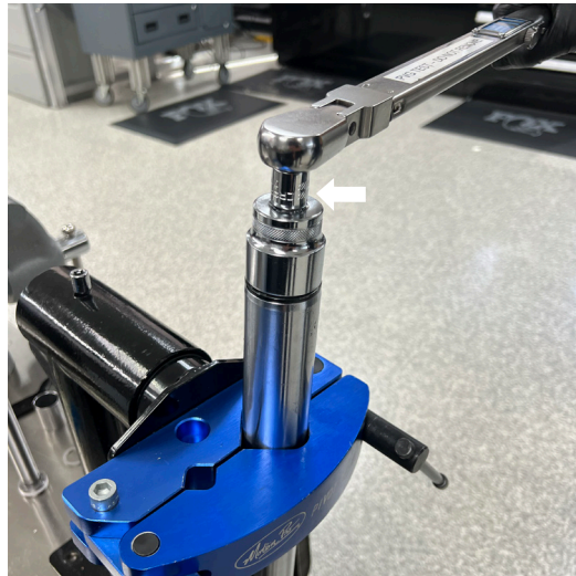
Fig. 26: Torque the top cap.
