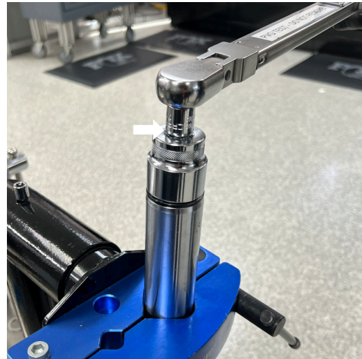
Fig. 19: Torque the top cap.
