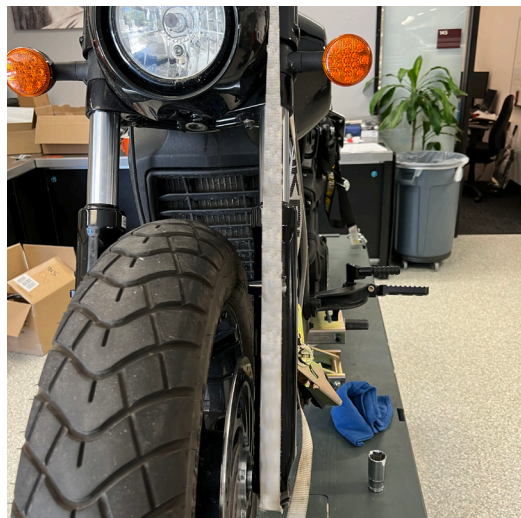
Fig. 28: Use of ratchet strap to compress fork for wheel installation.
