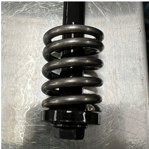
Fig. 11: Correct orientation of negative spring.
