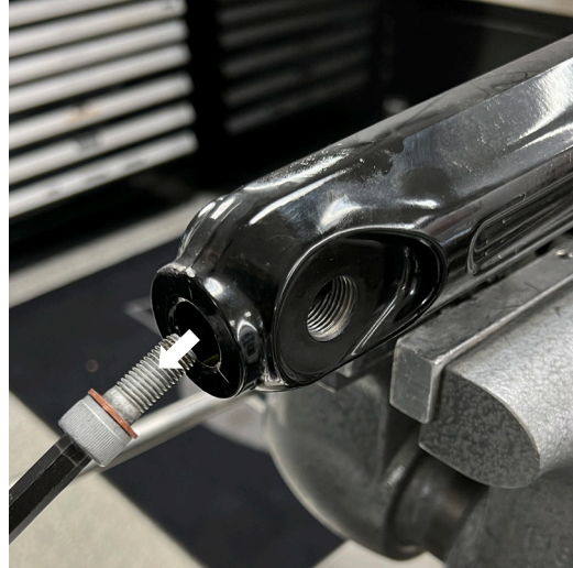
Fig. 6: Clamp the lower portion of the fork and remove the retaining screw.
