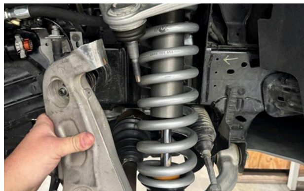
Fig. 2: Separate the steering knuckle.
