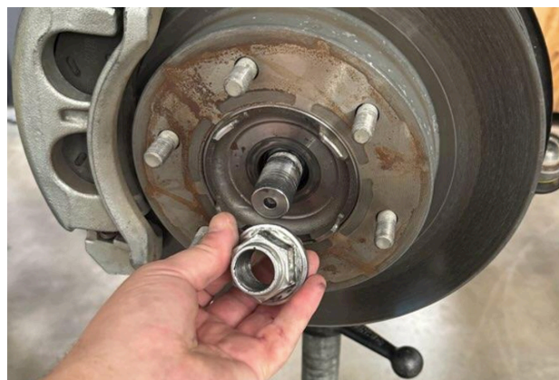
Fig. 3: Remove nut from drive shaft.
