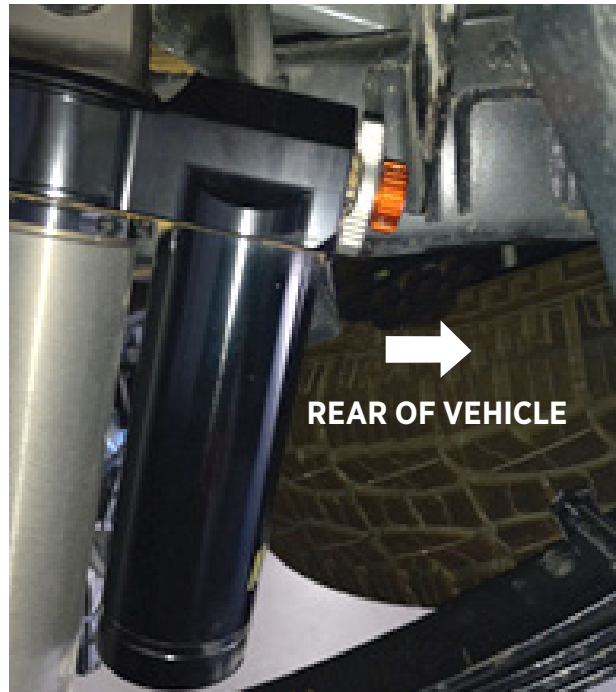
Fig. 11: Rear shock orientation (right side).
