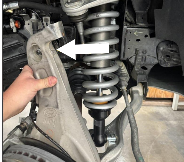
Fig. 4: Disconnect the sway bar link.
