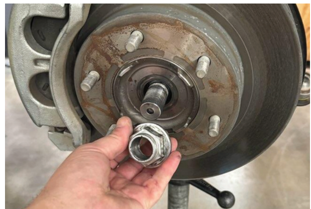
Fig. 3: Remove nut from drive shaft.
