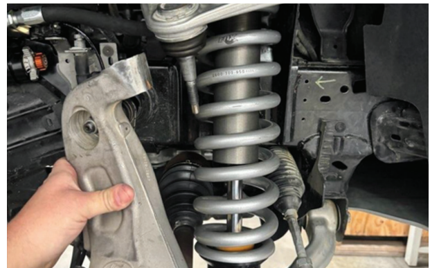
Fig. 2: Separate the steering knuckle.
