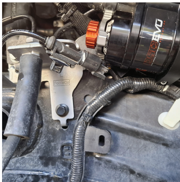
Fig. 12 ABS connector relocation.
