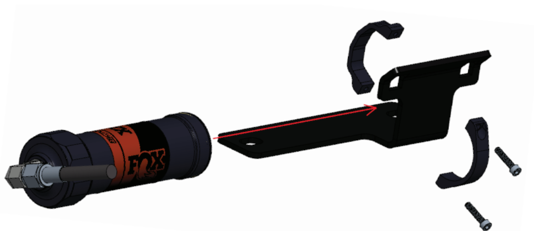
Fig. 12: Attach the reservoir bracket to the reservoir.
