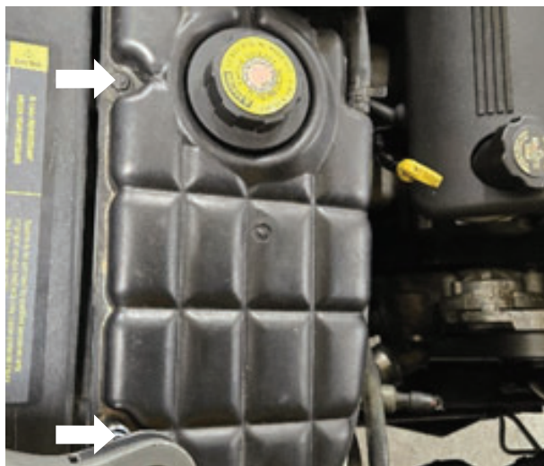
Fig. 1c: C5 model - remove fasteners.
