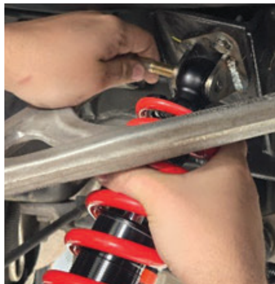
Fig. 34: Install the top eyelet to the mount.
