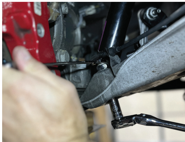
Fig. 5: Remove the lower shock bolts.
