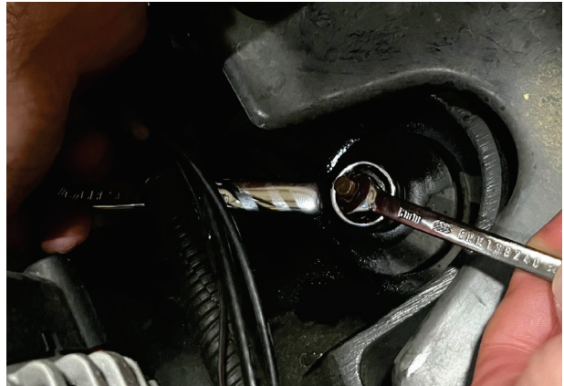
Fig. 2: Loosen the top shock mounts.
