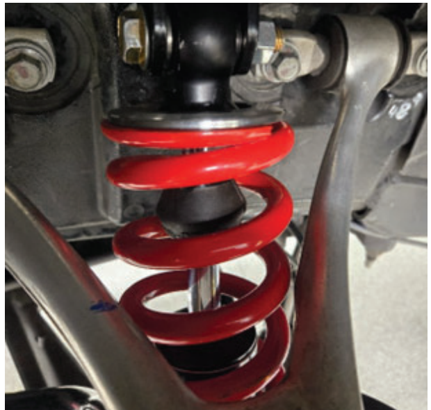
Fig. 16: Clearance between spring and UCA.
