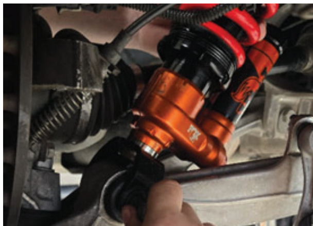
Fig. 33: Install the lower clevis.
