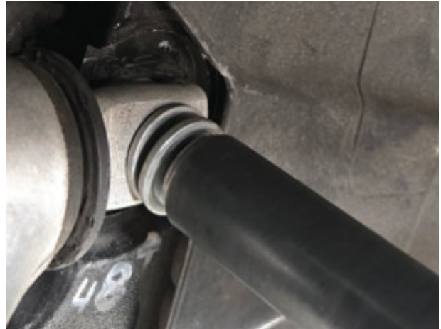
Fig. 15: Reinstall the UCA.
