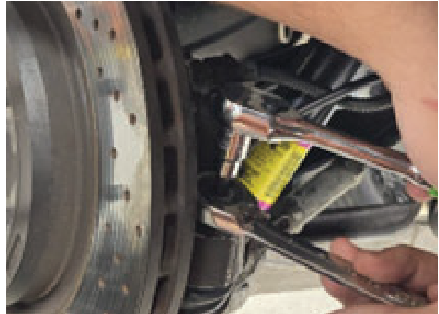
Fig. 20: Remove the toe link from the knuckle.
