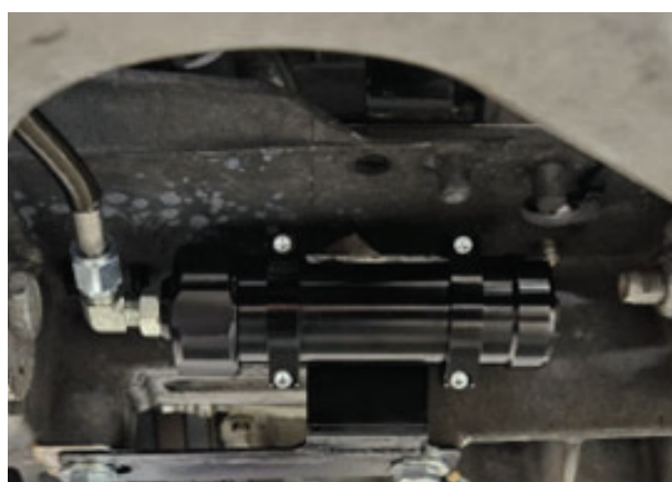
Fig. 18b: Align the reservoir in the center of the LCA mounts.
