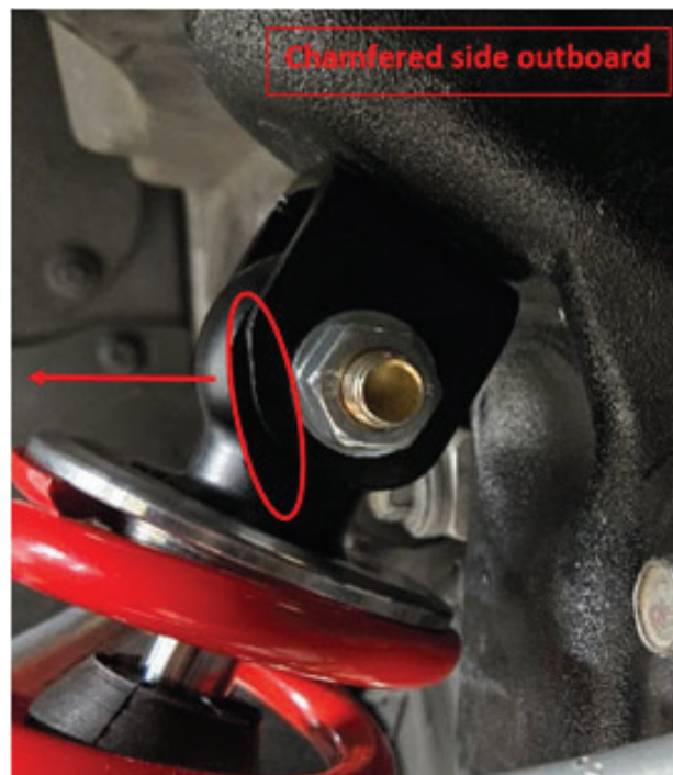
Fig. 14: Chamfer facing away from the chassis.
