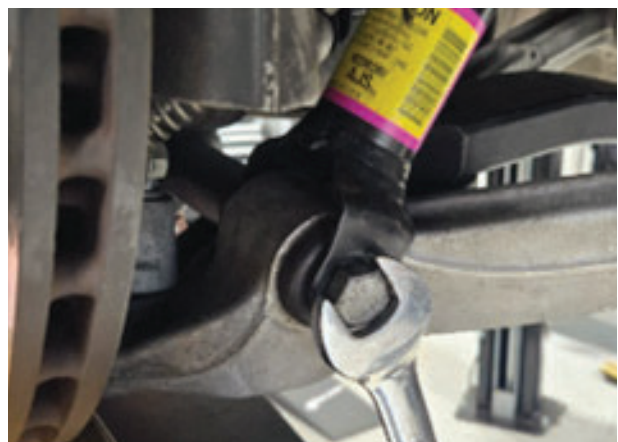
Fig. 22: Remove the lower shock bolt.
