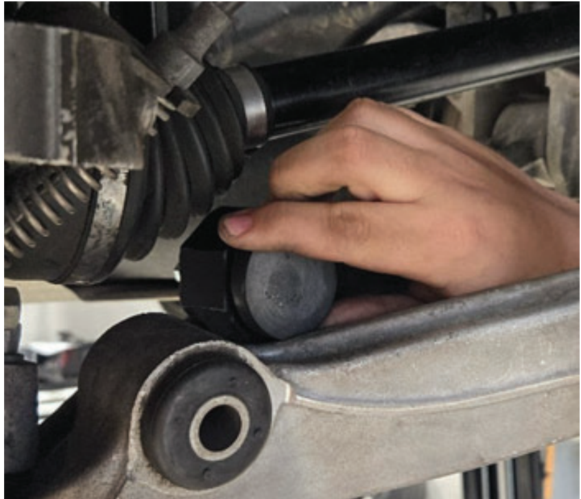
Fig. 27b: C6 model - remove the spring jacking bolts.
