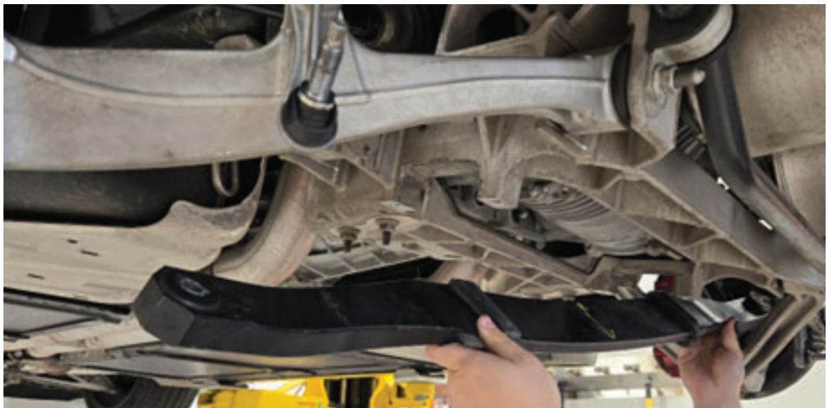
Fig. 27c: C6 model - remove the leaf spring.
