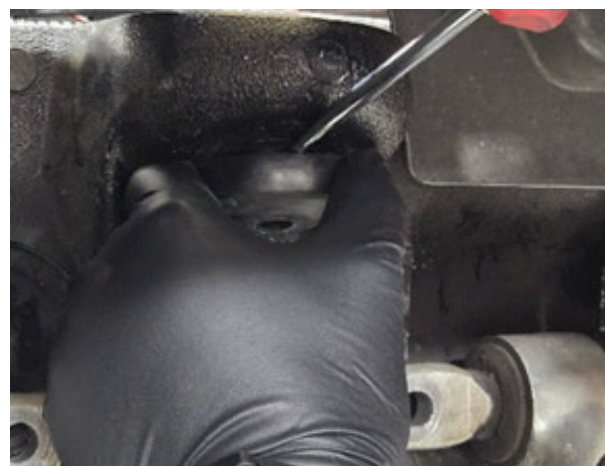
Fig. 8: Remove the upper shock bushing.
