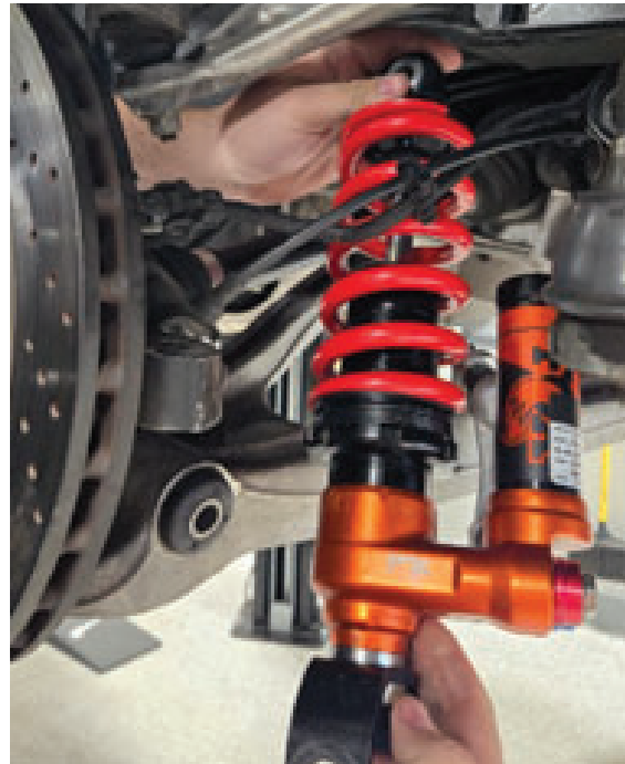
Fig. 32: Install the FOX shock with the adjusters facing toward the front of the vehicle.
