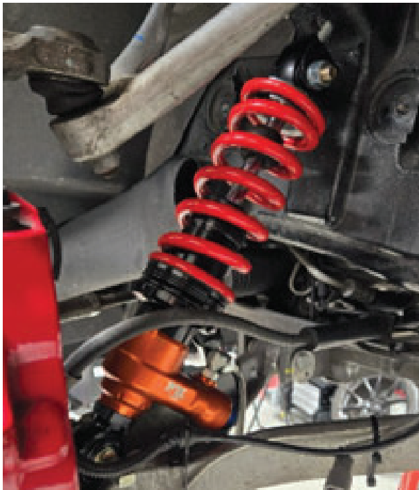
Fig. 13: Install the FOX shock.
