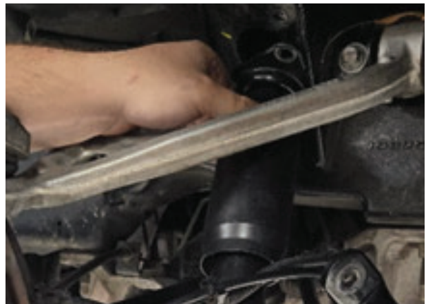
Fig. 24: Remove the stock shock.
