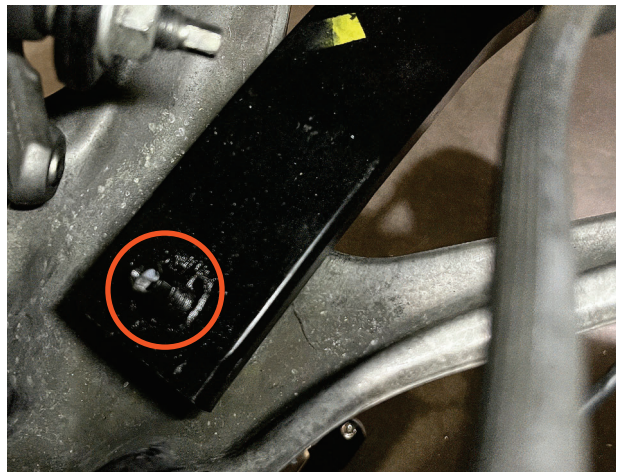
Fig. 3: Remove all preload (circled area).
