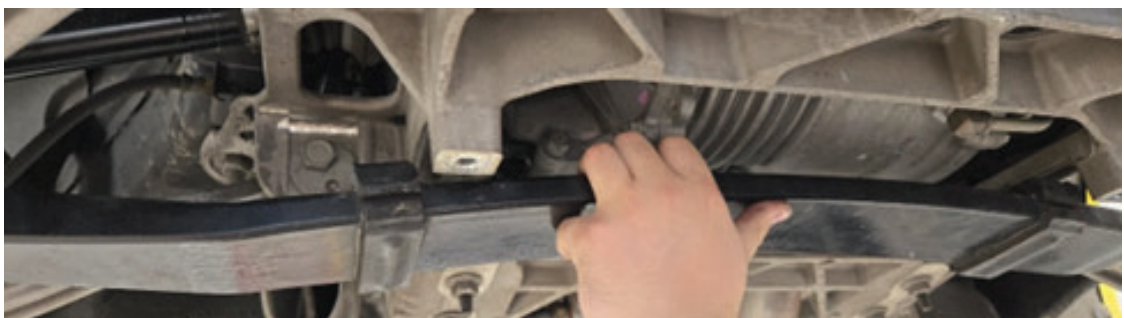
Fig. 27a: C6 model - rotate and slide the leaf spring.
