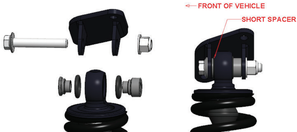
Fig. 30: C5 top mount and mounting hardware.
