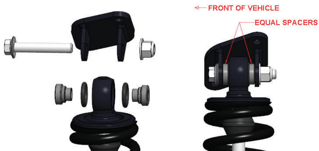
Fig. 31: C6 top mount and mounting hardware.
