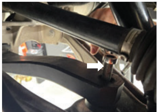
Fig. 25b: Turn the jacking bolts counter-clockwise.
