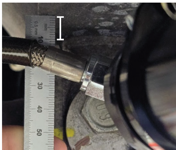
Fig. 19: Proper hose position and 10 mm clearance gap to chassis.
