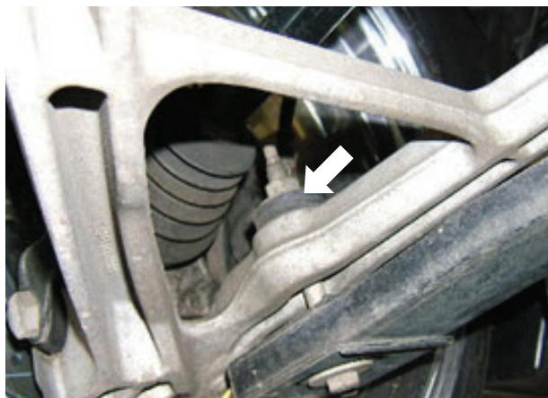
Fig. 25a: Remove the lockring ring.
