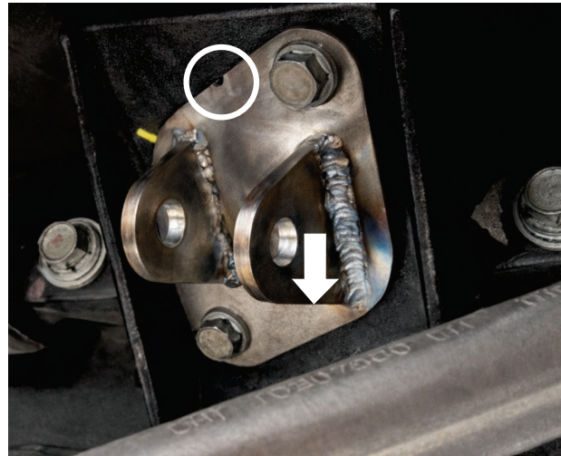
Fig. 29: Install the FOX top mount with the notch (circled area) oriented on the top, and the long edge of the tab (arrow) facing down.
