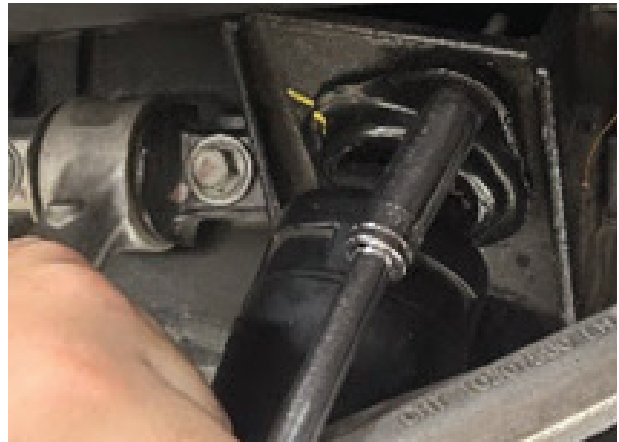
Fig. 23: Remove the upper shock bolts.
