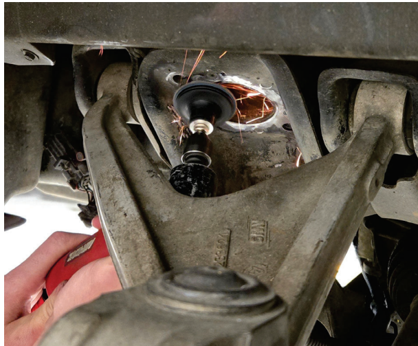
Fig. 28: Grind top mount surface (steel frame chassis only).
