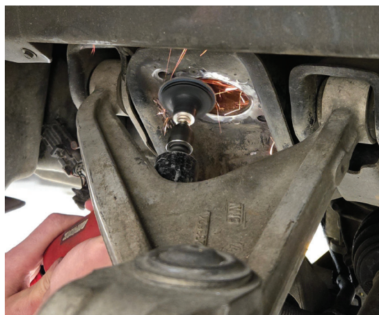
Fig. 11: Grind top mount surface (steel frame chassis only).
