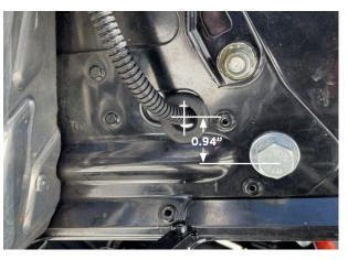
Fig. 4A: MY24 and older: Second mark for drilled hole Fig. 4B: MY25 and newer: Second mark for drilled hole
