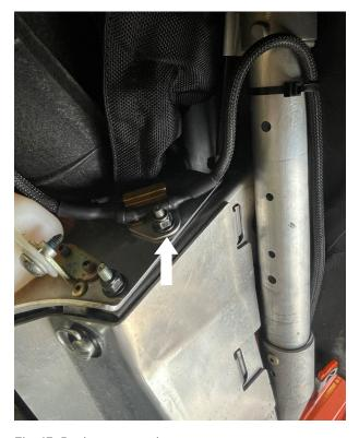
Fig. 13: Resistor mounting
