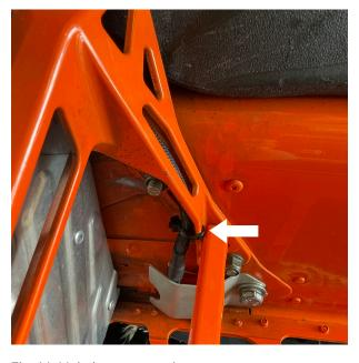
Fig. 14: Main harness routing
