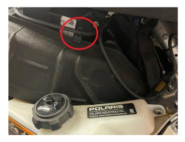
Fig. 15: Secure the harness routing clip
