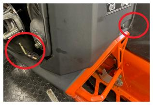
Fig. 1: Remove clutch tool and console screw
