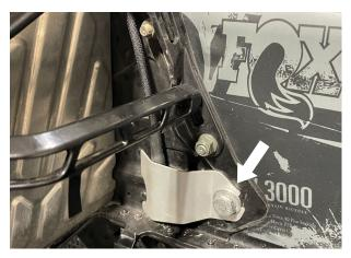
Fig. 12: Install wire guard
