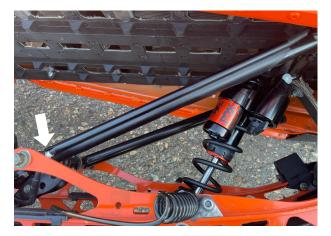
Fig. 8: Wire shield installation
