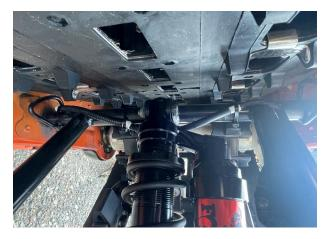
Fig. 10: Secure the harness to the pivot tube
