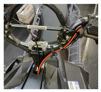
Fig. 21: Switch lead routing
