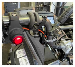
Fig. 20: Switch lead routing
