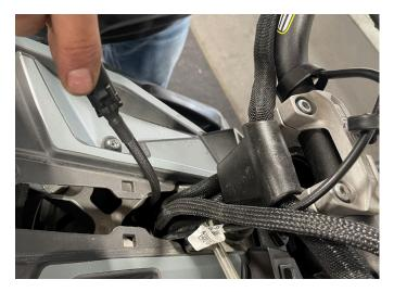
Fig. 16: Switch lead routing
