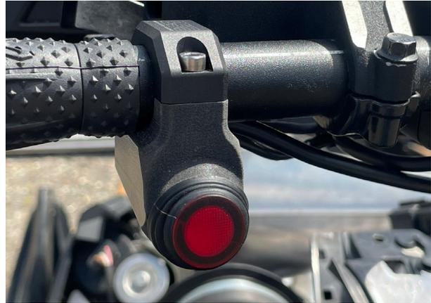
Fig. 17: Switch position under handlebar
