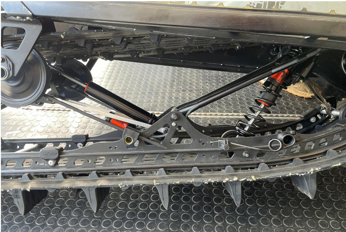
Fig. 4: Coil shock placement
