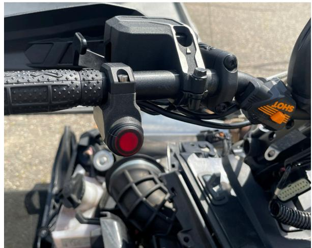
Fig. 18: Switch lead routing
