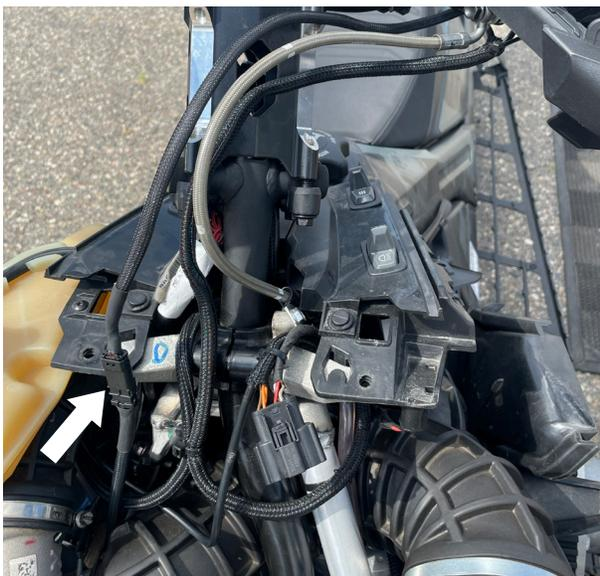
Fig. 19: Switch lead routing
