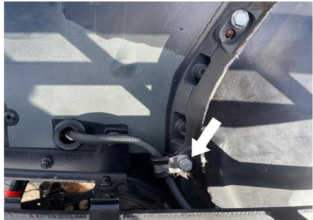
Fig. 11: Secure the harness routing clip.
