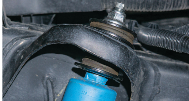
Fig. 10: Remove upper mounting hardware (reference image may look different than your upper mounting hardware, but same steps apply).
