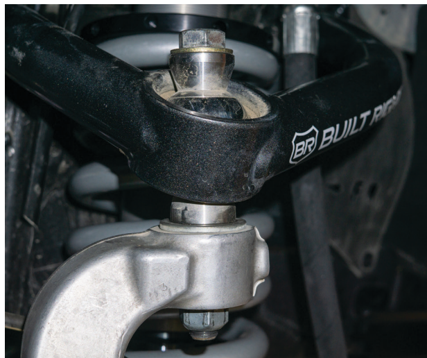
Fig. 7: Reattach UCA to the upright.
