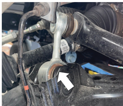
Fig. 2: Sway bar end link (reference image may look different than your end link, but same steps apply)
