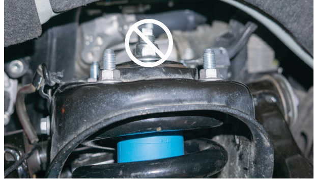
Fig. 4: Remove the top hat nuts. Do NOT remove the center nut.
