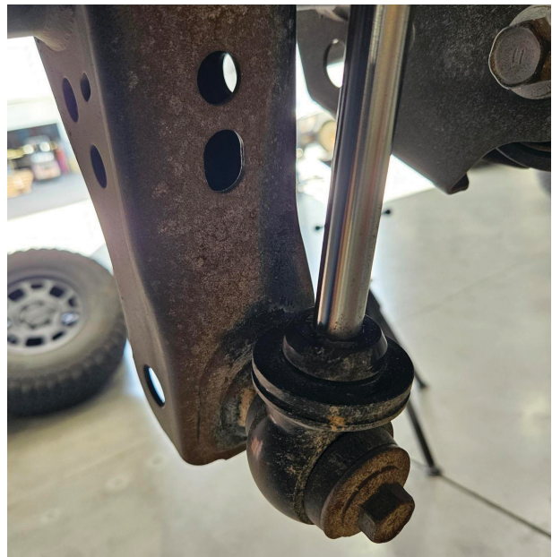
Fig. 14: Install the lower shock bolt (passenger side shown).
