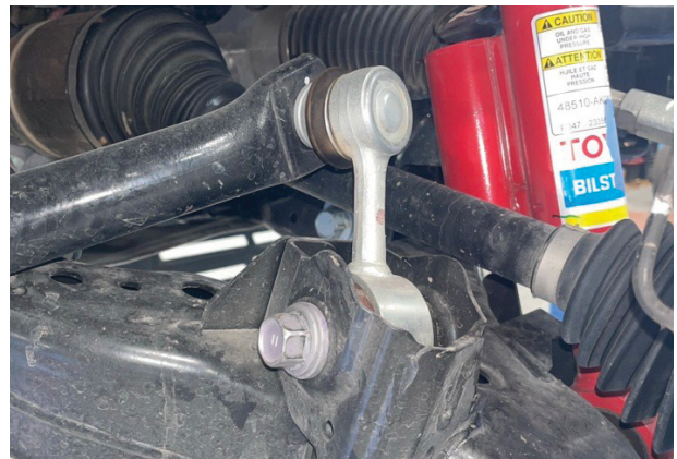
Fig. 9: Sway bar end link (reference image may look different than your end link, but same steps apply)
