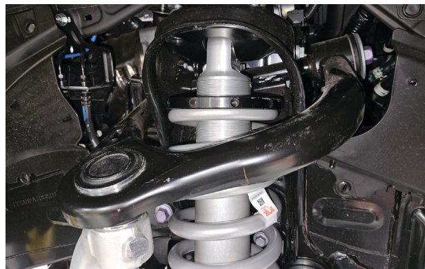
Fig. 6b: The side with the nitrogen port faces inboard.
