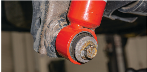
Fig. 11: Remove lower mounting hardware (reference image may look different than your lower mounting hardware, but same steps apply).
