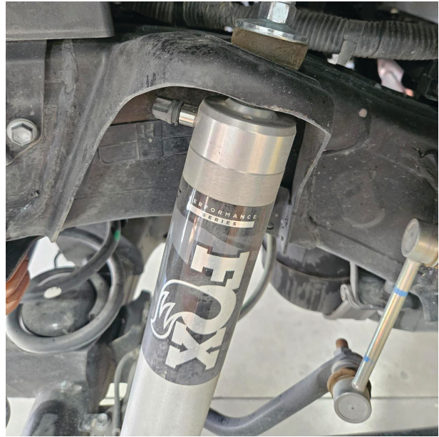
Fig. 12: Install the shock with the logo pointed outward.
