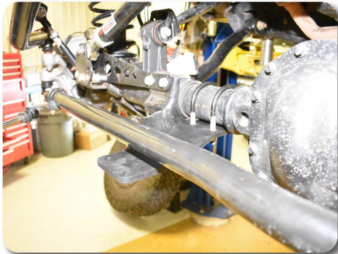
4. Attach the driver's side stabilizer bracket to the bottom side of the tie rod next to the clamp (Fig. 2) with the provided 5/16" U-bolts, washers, and nuts so the stabilizer mounting hole offsets to the outside. Leave hardware loose. Bolt Pack 304
