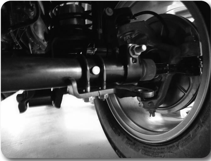
5. Loosely attach the passenger side stabilizer bracket to bottom side of tie rod link similar to the driver side with the provided 5/16" U-bolts, washers, and nuts. Leave hardware loose. Bolt Pack 304
