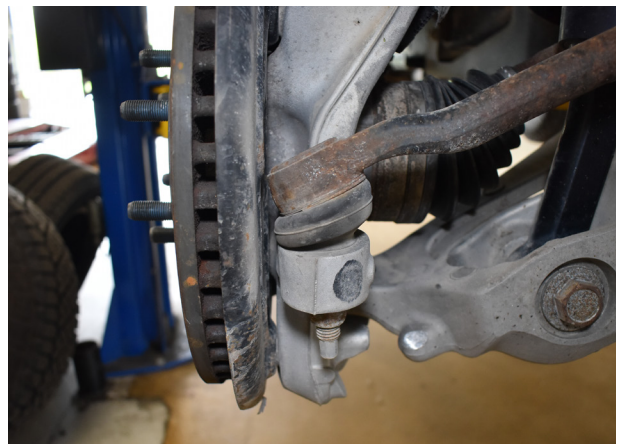
Figure 1: Disconnect tie rod.
