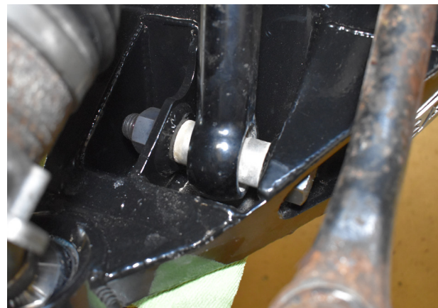
Figure 18: Install nylock nut and washer.
