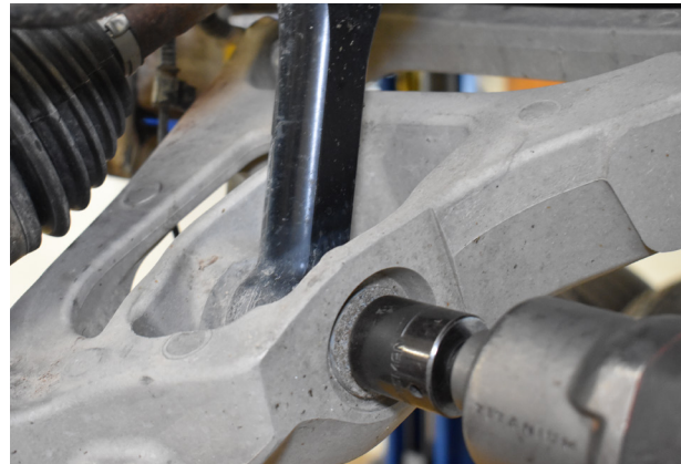
Figure 6: Remove lower strut bolt.
