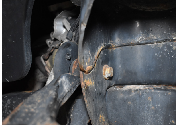
Figure 8A: Remove the UCA bolt and nut.
