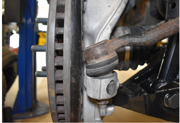
Figure 19: Install nylock nut and washer.
