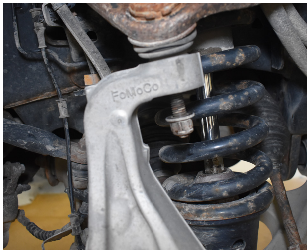
Figure 4B: Loosen ball joint nut.
