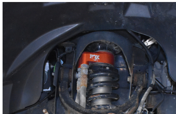
Figure 7: Remove the 3 top strut nuts.
