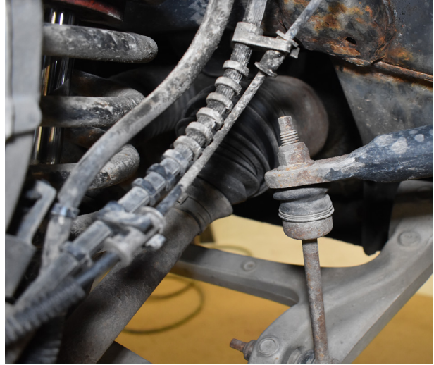
Figure 3: Disconnect ABS lines.
