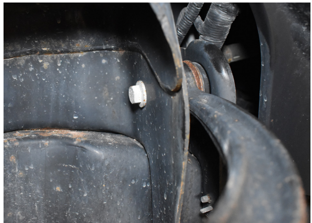
Figure 8B: Remove the UCA bolt and nut.
