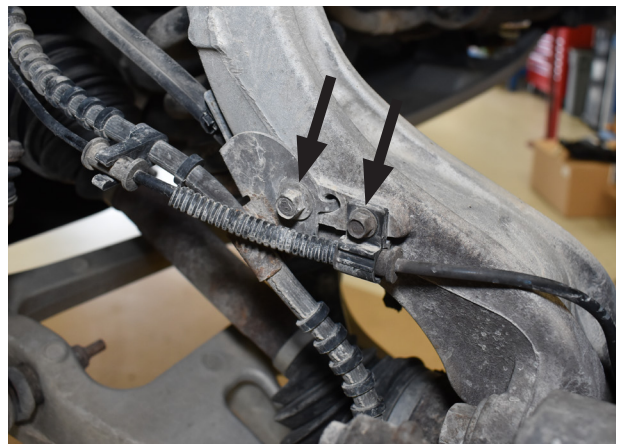
Figure 2: Disconnect brake line bracket.
