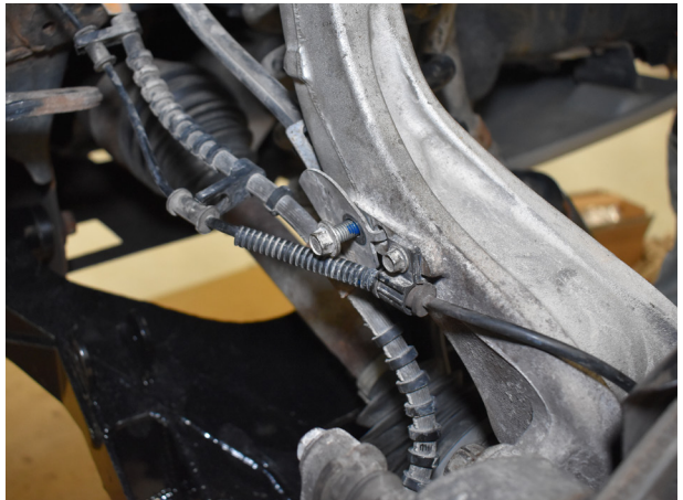
Figure 20: Re-attach ABS and brake line brackets.
