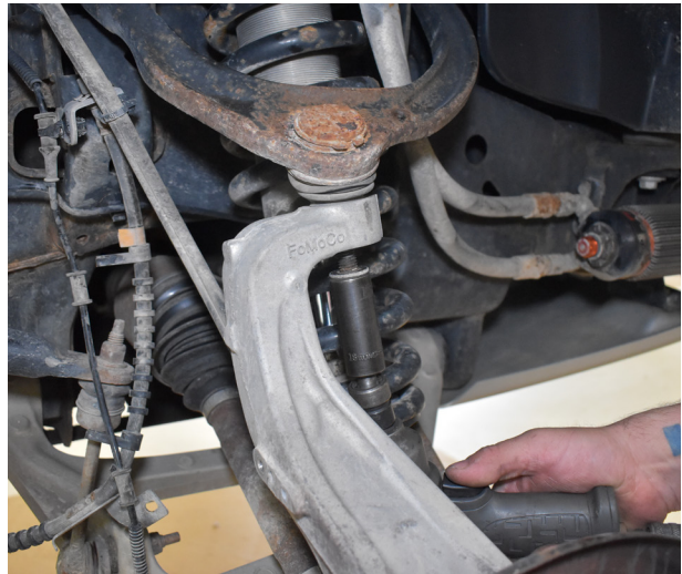
Figure 4A: Loosen ball joint nut.
