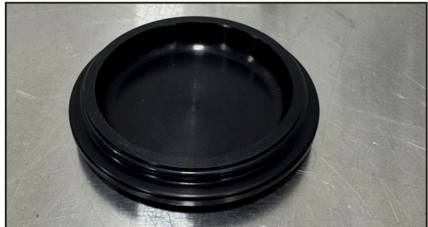
Fig. 15: Install O-Ring into cap groove.
