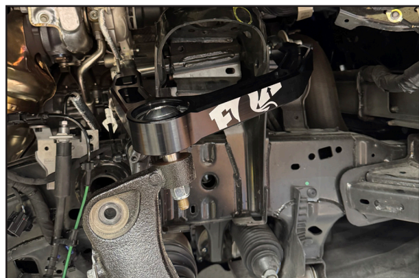
Fig. 12: Install misalignment into knuckle.
