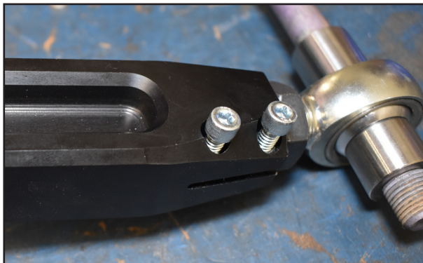
Fig.7: Install pinch bolts.
