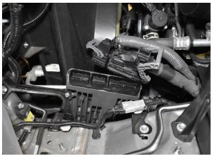
Fig. 7: PCM harness connector 3.
