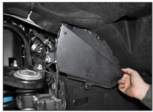
Fig. 11: Brake line shield removal
