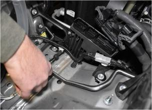
Fig. 8: Remove 3 harness clips.
