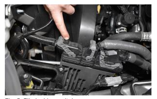
Fig. 5: Flip locking switches.
