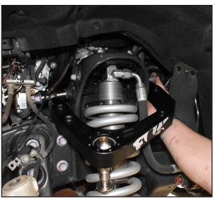
Fig. 22: Install Upper Control Arm.
