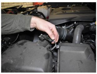
Fig. 1: Disconnect wire harness
