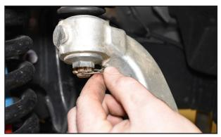
Fig. 13: Remove cotter key.
