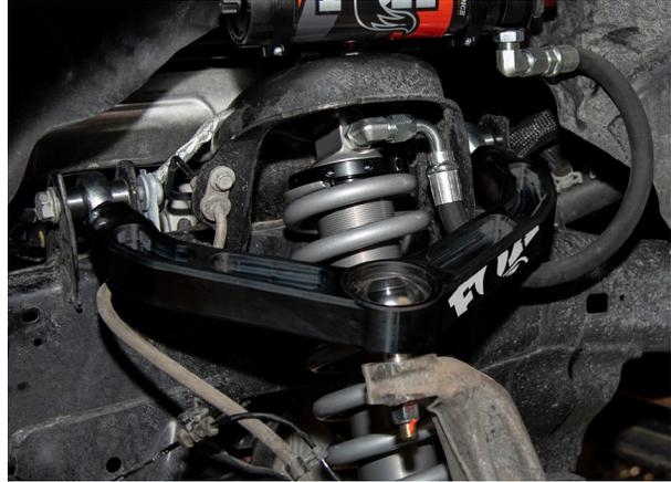
Fig. 17: Install upper control arm.
