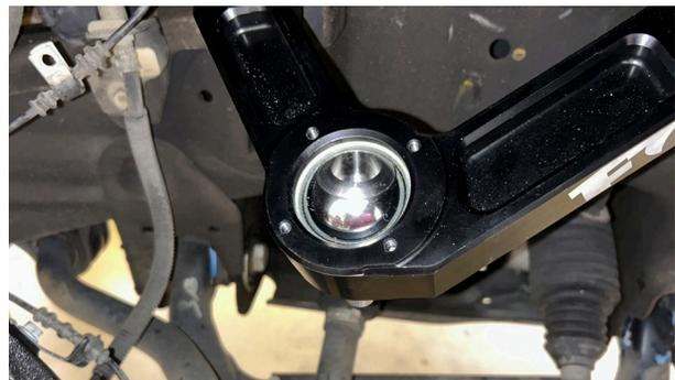
Fig. 16: Assemble uniball joint.
