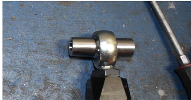
Fig. 14: Install misalignments.
