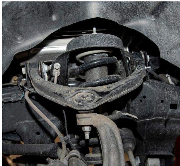
Fig. 1: Disconnect upper control arm from knuckle.
