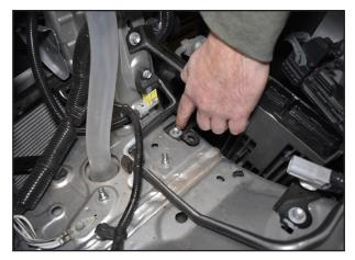
Fig. 9: Remove PCM bolts
