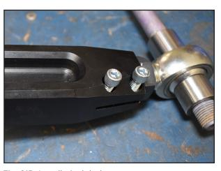
Fig. 21B: Install pinch bolts.
