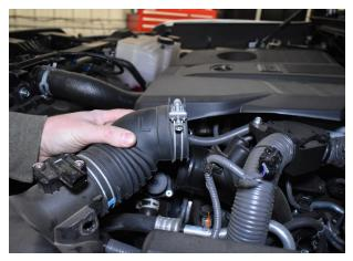
Fig. 2: Loosen the air hose clamp
