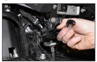
Fig. 12B: Loosen UCA hardware.
