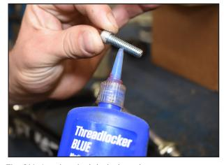
Fig. 21A: Loctite pinch bolt threads.
