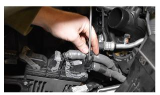
Fig. 4A: Remove PCM Clip.
