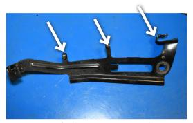
Fig. 24A: Bend tabs to remove ABS line.
