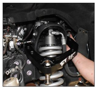
Fig. 22: Install Upper Control Arm.
