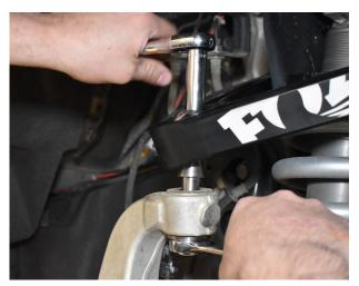
Fig. 23: Attach Upper Control Arm to knuckle.
