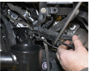
Fig. 24B: ABS line bracket.
