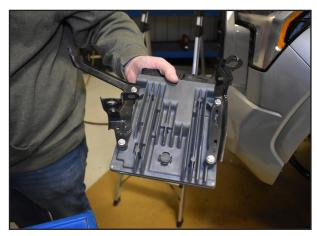
Fig. 10: Remove PCM.
