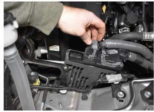
Fig. 6: PCM harness connector 2.
