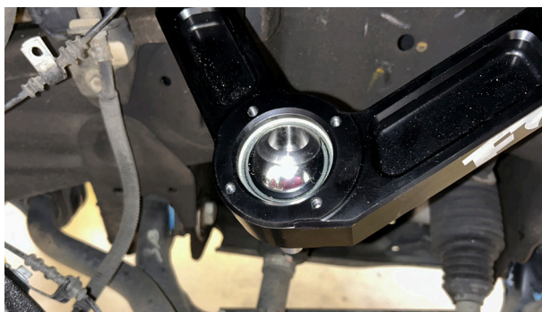
Fig. 16: Assemble uniball joint.
