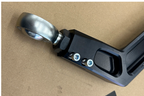
Fig. 13: Loctite and install pinch bolts.
