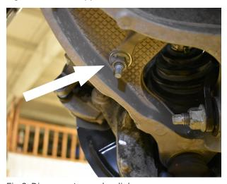
Fig.2: Disconnect sway bar link.
