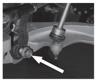
Fig. 5: Lower strut nut and bolt.
