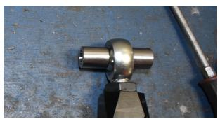
Fig. 14: Install misalignments.
