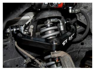
Fig. 17: Install upper control arm.
