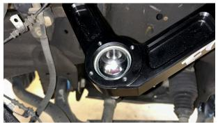
Fig. 16: Assemble uniball joint.
