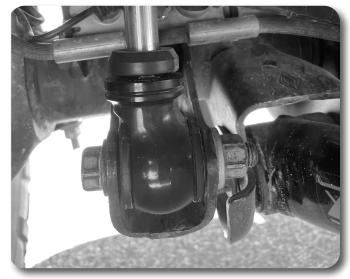
5. Tighten upper mount hardware to 80 ft-lbs and lower mount hardware to 75 ft-lbs.
