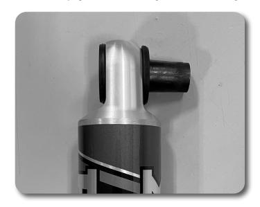
4. The lower mount will be installed with the shaft offset away from the body, as shown below.
